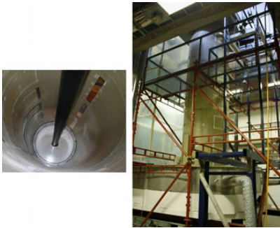
Fig. 1 Picture of 6 m high natural convection rig: outside (right), inside (left) showing heated cylinder.
