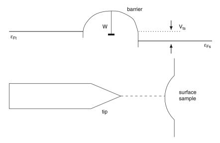
Fig. 4.8 Scanning tunneling microscope
