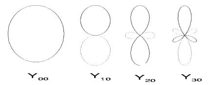
**Fig. 5.2** Projection of the spherical harmonics  $Y_{l0}$  on the (x,z) plane, for the values l=0-3. While all the  $Y_{l0}$  are axially symmetric wave functions, l=0 implies full spherical symmetry. The distance from the *center* to the *top* of the figures is  $\sqrt{(2l+1)/4\pi}$ . *Solid lines* denote positive lobules; *dotted lines*, negative ones
