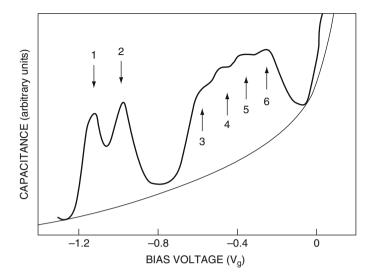
Fig. 7.5 Capacitance spectroscopy reveals quantum-dot electron occupancy and ground-state energies. (Reproduced with permission from [45])
