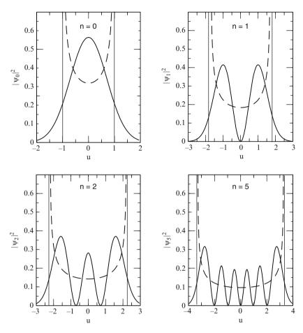
**Fig. 4.2** Quantum mechanical probability densities and the classical probability densities of a harmonic oscillator potential as a function of the dimensionless distance u, for the quantum numbers n = 0, 1, 2 and 5. *Vertical lines* represent the limits of the classically allowed interval
