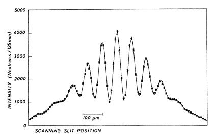
**Fig. 2.6** A double-slit diffraction pattern measured with neutrons (Reprinted from [78]. Copyright by the American Physical Society and the Institut für Experimentalphysik, Universität Wien)
