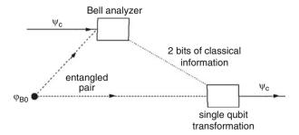
Fig. 13.1 Scheme illustrating the process of teleportation. *Dashed lines* represent entangled qubits in the state  $\varphi_{B_0}$ , while the *dotted line* indicates that classical information is transmitted
