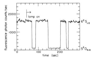
Fig. 12.4 Quantum jumps of a single ion in a trap. (Reprinted with permission from Nagourney et al. [85], with authorization from the American Physical Society)
