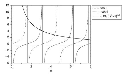
Fig. 4.5 Graphical determination of the energy eigenvalues of a finite square well potential. The intersections of the *continuous curve*  $\sqrt{(13/\theta)^2 - 1}$  with the *dashed curves* correspond to even-parity solutions, while those with the *dotted curves* correspond to the odd ones. The value  $MV_0a^2/\hbar^2 = 338$  is assumed
