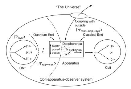
**Fig. 14.2** Sketch of the measurement of a qubit. "Rest" is called "environment" in the text. Initially, there is a superposition of the two nuclear states. One of the two alternatives for the Schrödinger cat occurs at the classical end. (Reproduced from J. Roederer [20], with permission from Springer-Verlag)
