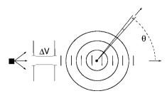
Fig. 6.2 Schematic representation of a scattering experiment. After being produced in a source, the projectile is collimated, accelerated and collimated again. It collides with the target in the form of a plane wave. It is subsequently scattered as a spherical wave, within a solid angle that makes an angle  $\theta$  with the direction of incidence
