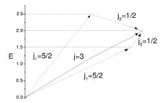
**Fig. 5.5** Coupling of two vectors with  $j_1 = 5/2$  and  $j_2 = 1/2$  (dotted lines) may yield a vector with j = 3, m = 2 (continuous line). The superposition (5.31) has two components, with  $m_1 = \frac{3}{2}$ ,  $m_2 = \frac{1}{2}$  and  $m_1 = \frac{5}{2}$ ,  $m_2 = -\frac{1}{2}$ , respectively
