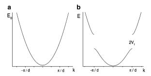
Fig. 8.5 Bands in periodic potentials. The unperturbed parabolic energies are given as functions of k in (a). The eigenvalue  $E_-$  is plotted in the interval  $0 \le |k| \le \frac{\pi}{d}$  and  $E_+$  for  $\frac{\pi}{d} \le |k|$  in (b)
