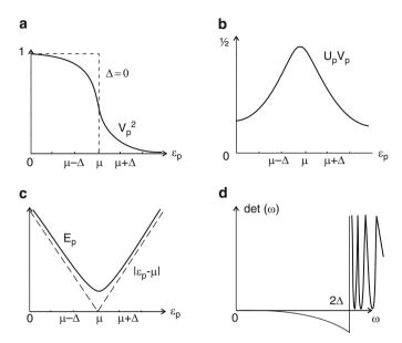
**Fig. 10.1** Occupation probabilities  $V_p^2$  (**a**); amplitudes  $U_pV_p$  (**b**); and quasi-particle energies  $E_p$  (**c**), as functions of the particle energies  $\epsilon_p$ . The determinant  $\det(\omega)$  is represented as a function of  $\omega$  in (**d**) [see (10.29)]
