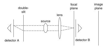
Fig. 12.2 A double-slit diffraction pattern measured with entangled photons. The two photons are detected after the double slit and at the focal plane of the lens, respectively. Detector B may also be displaced towards the image plane
