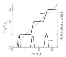
**Fig. 7.8** The integer quantum Hall effect appears as plateaus in the Hall resistivity of a sample which coincide with the disappearance of the sample's electrical resistivity, as the magnetic field strength is varied [51]. (Reproduced with permission from Springer-Verlag)
