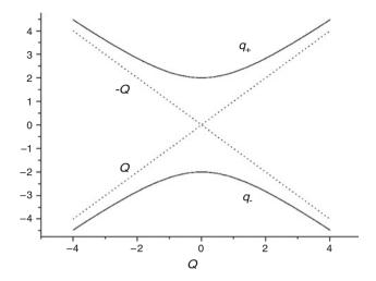
Fig. 3.1 Eigenvalues  $q_{\pm}$  of a 2 × 2 system (continuous curves) as functions of Q, half of the energy distance between the diagonal matrix elements (dotted lines)
