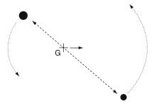
**Fig. 8.3** Vibrational (dashed line), rotational (dotted lines) and translation of the center of mass G (continuous line) of a diatomic molecule
