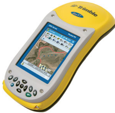
Fig. 14.1 Mobile hand-held GNSS. Source ©1995–2010 ESRI. http://www.esri.com/technology-topics/mobile-gis/graphics/geoxt-web-lg.jpg
