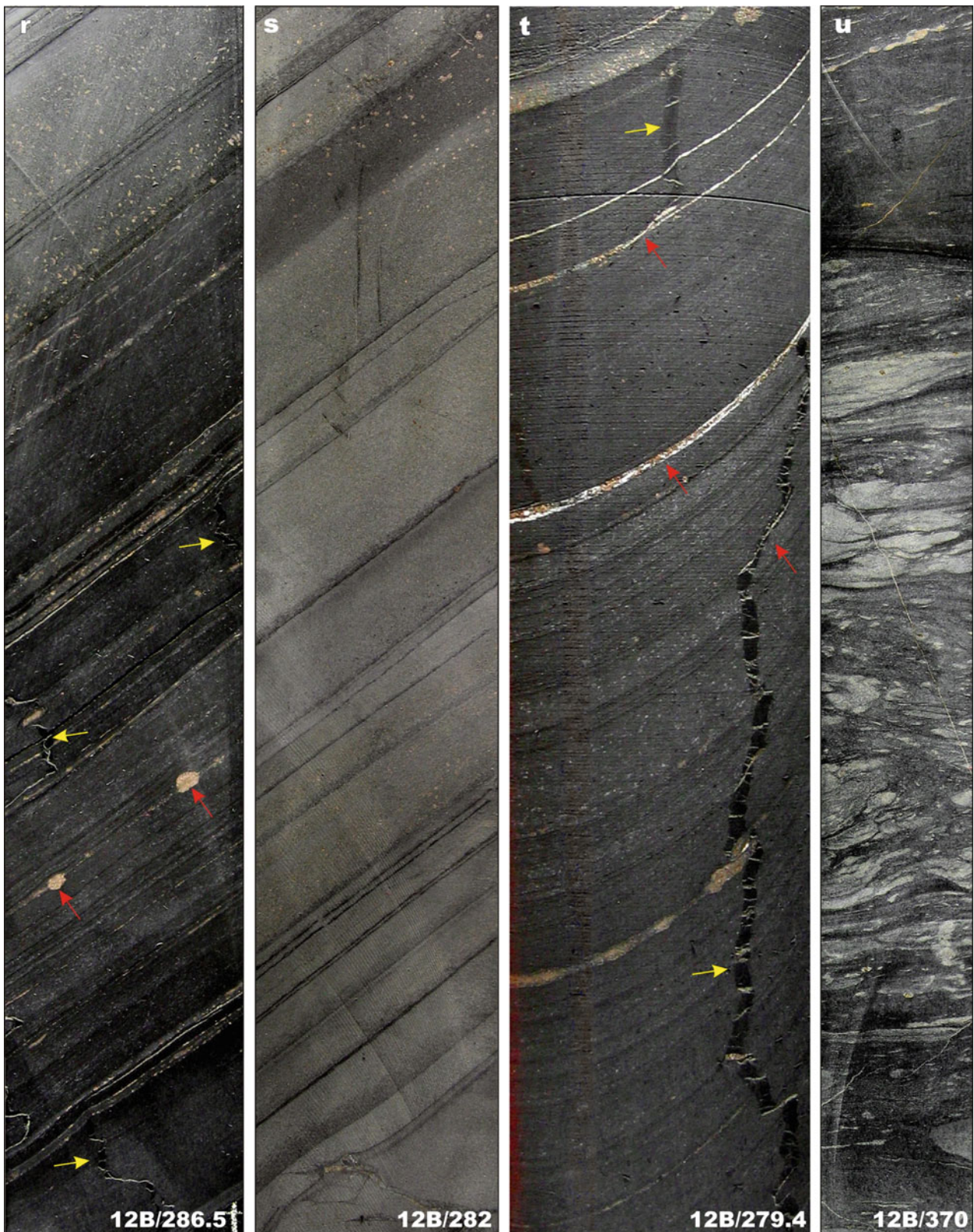
Fig. 4.52 (continued) (r) C_{org} -bearing, parallel-laminated siltstone with thin pyrobitumen-rich veins (yellow arrowed) and small sulphide nodules (red arrowed). (s) Rhythmically bedded greywacke-siltstone. (t) Parallel-laminated siltstone with pyrobitumen-rich vein
