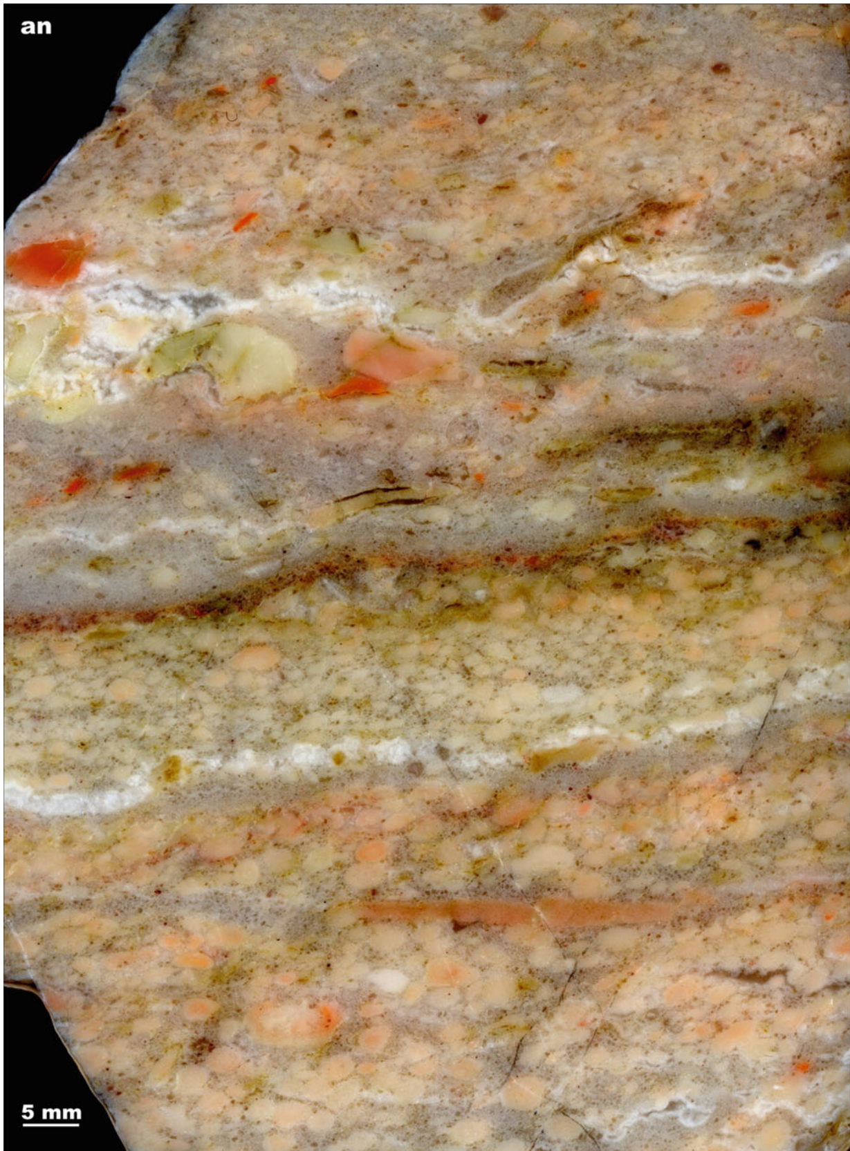
Fig. 4.21 (continued) (an) Polished slab exhibiting crudely bedded, allochemical dolostone; uniform, sub-spherical dolomite particles in the lower part may represent recrystallised oolites, whereas clasts in the upper bed range in size, shape and composition, and represent
