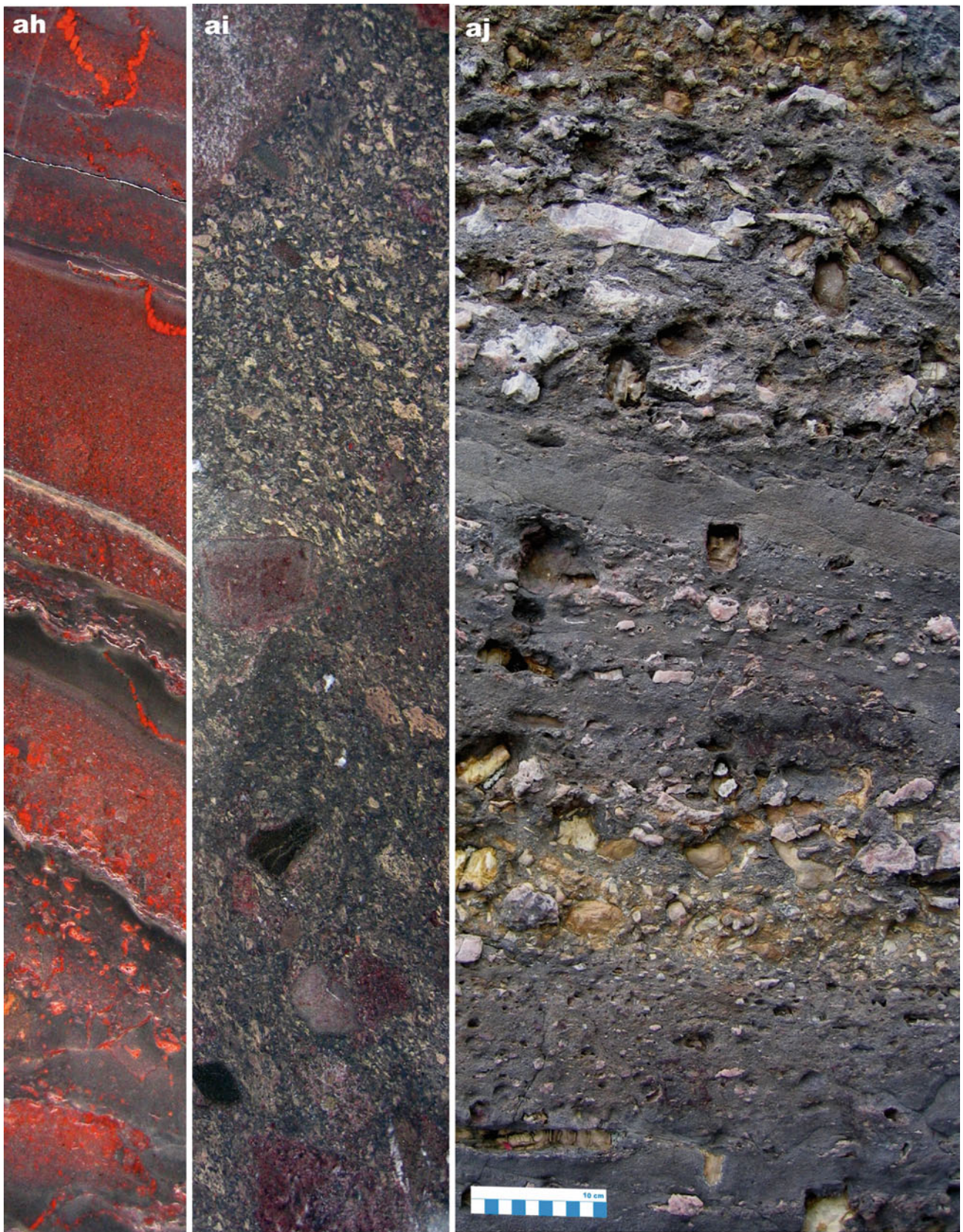
Fig. 4.26 (continued) (ah) A series of jasper sandstone grading into brown siltstone intersected by jasper veinlets. (ai) Tuff composed of unsorted clasts of intensively altered ferropicritic lava in psammitic ferropicritic tuff matrix; core diameter is 5 cm. (aj) Cross-section view
