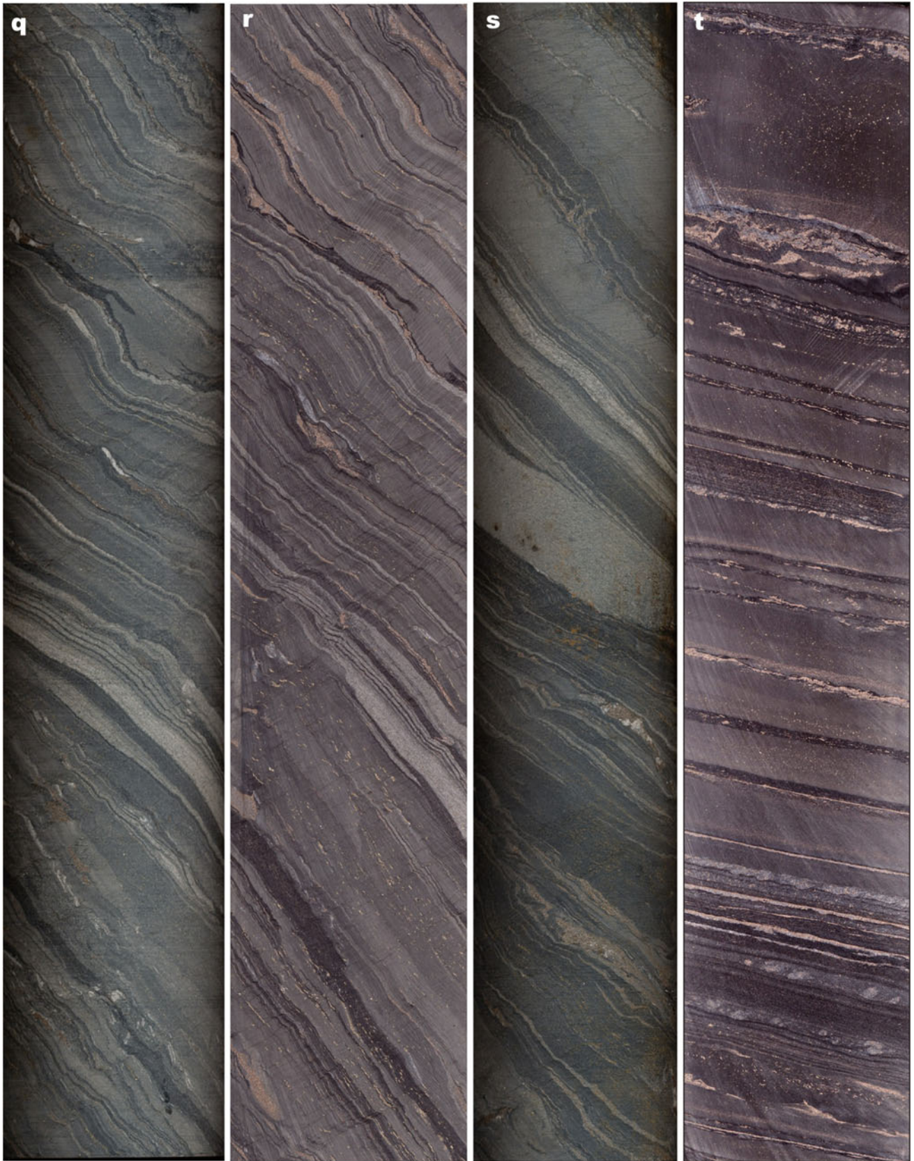
Fig. 4.29 (continued) (q, r, s) Thinly-laminated sandstone-siltstone with rare mudstone units; some light-coloured sandstone beds have an erosive base. (t) Rhythmically- and parallel-bedded siltstone-mudstone; siltstone exhibits faint grading. Core diameter is 6 cm
