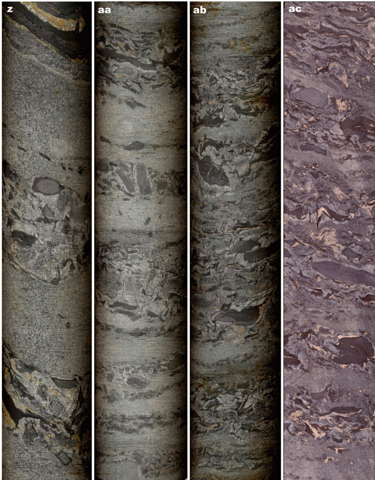
Fig. 4.29 (continued) (z) Interbedded, massive greywacke and calcite-cemented breccia capped by black mudstone bed on top; fragments in breccia beds are mainly angular, soft-sediment-deformed, black mudstone and greywacke. (aa) Rhythmic interbedding of massive sandstone and breccia composed of dismembered and soft-sediment-deformed mudstone and greywacke cemented by calcite. (ab)
