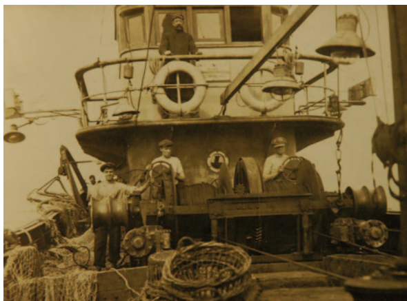
Fig. 10.1 Crew on aft deck with net and stem winches on a State Trawler, 1914–1921. Courtesy State Library of New South Wales. (David G. Stead; [ML MSS 5715 11(25)])
