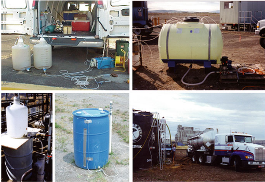
Fig. 2.1 Field push-pull test photographs showing various methods used to prepare and inject test solutions. Clockwise from upper left : separately prepared tests solutions in 50 L plastic carboys being combined and injected into a well using a peristaltic pump; 500 L test solution prepared in plastic tank; 240,000 L test solution being transferred from tanker truck to large plastic tank prior to injection; test solution in 200 L plastic drum being injected into monitoring well using a siphon; 50 L test solution in plastic carboy being injected into monitoring well by gravity drainage
