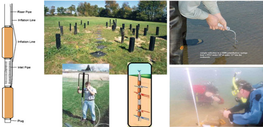
Fig. 1.2 Push-pull tests may be conducted (clockwise from top center ) using conventional monitoring wells, syringes and needles and temporary well screens in submerged sediments, in multi-level samplers, in drivel-point wells and in wells equipped with “straddle packers” to isolate a portion of the well screen to allow depth-specific testing
