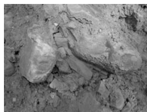
Fig. 3 The large quartz sandstone in the upper layer of profile, well rounded
