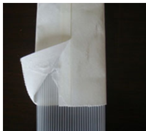
Fig. 4 Filter membrane of traditional PVD
