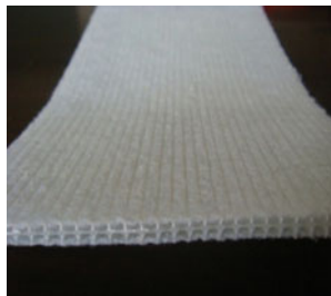
Fig. 3 Filter membrane of less clogging PVD
