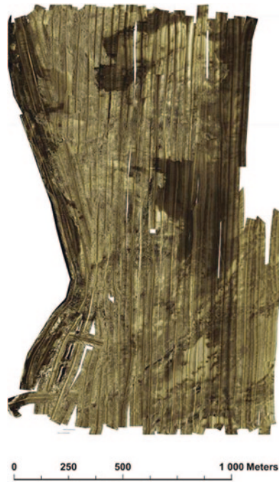
Fig. 4 Mosaic from SSS data with the spatial resolution of 0.1 m obtained by Coda Octopus software
