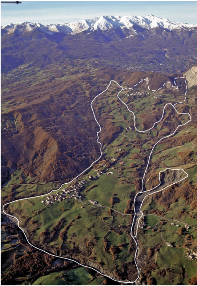
Fig. 3 The Large Morsiano landslide represents at the best the typical features of large earth flows; despite its age (a wood sample found inside it dates back to 13,500 Cal. years BP) the landslide is still active in several portions, threatening and damaging the village; according to historical records, reactivations occurred in 1631 (partial), 1651 (total), 1880 and 1959 (partial). (Photo by G. Bertolini, 2007–2008)
