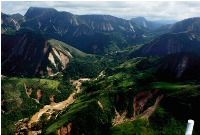
Fig. 1 Aerial view of some landslides which occurred on January 12th, 2011 in the mountainous region of Rio de Janeiro State where shallow translational landslides were dominant
