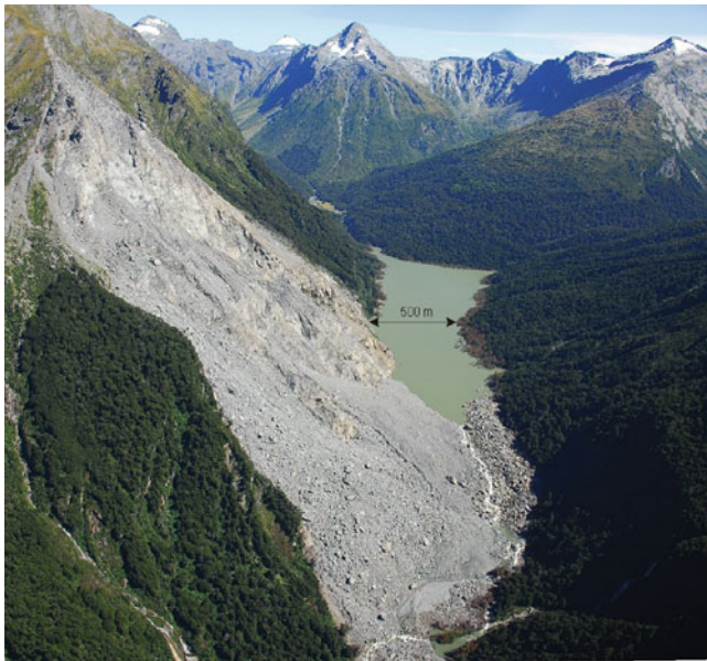
Fig. 4 Aerial view of Young River landslide. Note highly fractured rock mass at the apex of source area and fine textured talus apron which overlaps onto coarse debris at toe adjacent to lake. Lobes in fine textured debris suggested that the debris was saturated when it fell on 29 August 2007. Note also minimal snow persisting in catchment headwaters in late summer (Photo: GT Hancox)
