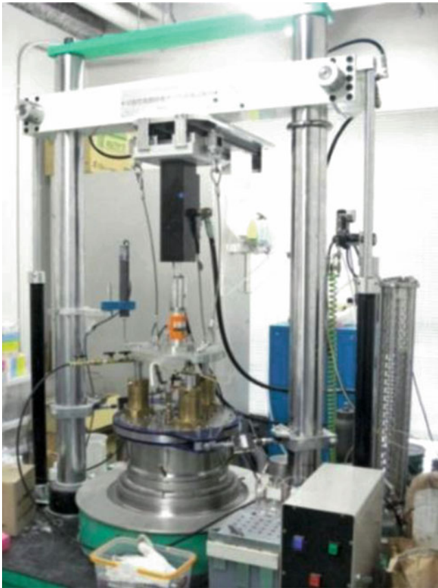
Fig. 4 Frontal view of the employed ring shear apparatus DPRI-7
