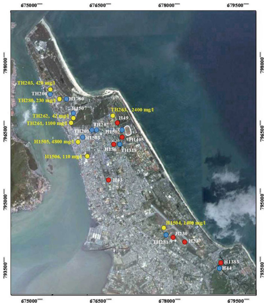
Fig. 8.6 Locations of available boreholes ( Yellow = \text{Cl}^- (shown here), TDS value (not shown, see Table 8.5) and screen interval; Red = lithology information; Blue = only screen interval)
