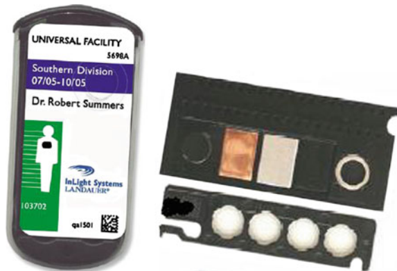
Fig. 10.3 The Landauer InLight ® dosimeter holder and detector slide (Courtesy of Landauer, www.landauer.com )
