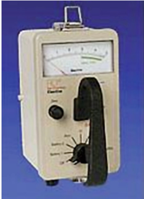
Fig. 11.1 Ionization survey instrument Model RO-20 offered by Thermo Fisher Scientific (Courtesy of Thermo Fisher Scientific, www.thermofisher.com )
