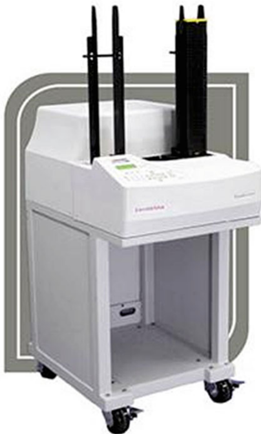
Fig. 11.14 The Canberra series 5E automatic low background alpha/beta counting system (Courtesy of Canberra, www.canberra.com )
