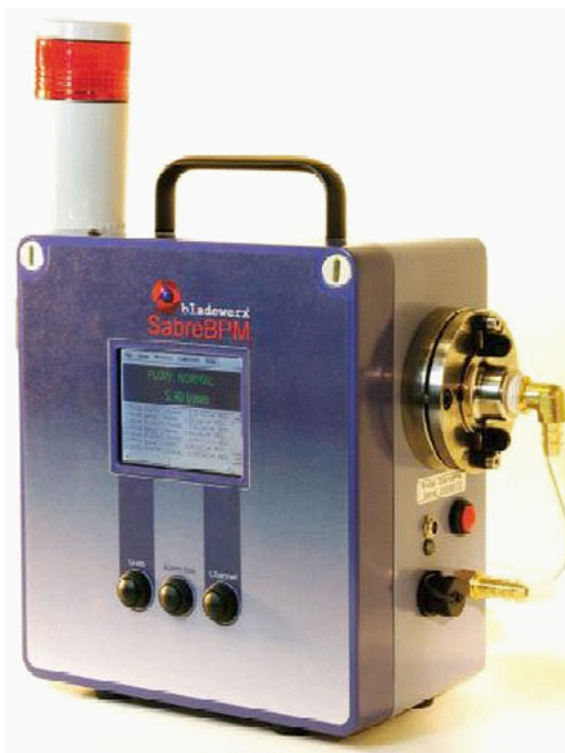
Fig. 11.21 The Bladewerx SabreBPM™ beta particulate monitor (Courtesy of Bladewerx, www.bladewerx.com )
