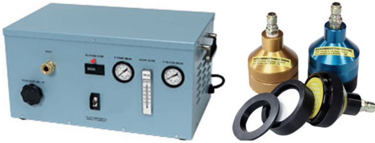
Fig. 6.12 The HI-Q self contained continuous duty air sampling unit and filter holders (Courtesy of HI-Q Environmental Products Company www.hi-q.net )
