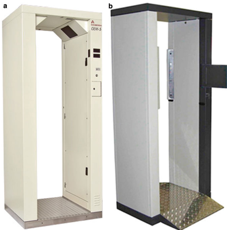
Fig. 6.16 Examples of portal, gamma-sensitive contamination monitors. a is the GEM TM -5 model offered by Canberra (Courtesy of Canberra www.canberra.com ). b is the PM-12 model offered by Thermo Fisher Scientific (Courtesy of Thermo Fisher Scientific, www.thermofisher.com )
