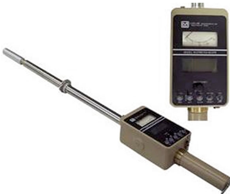
Fig. 11.5 Ludlum stretch scope dose rate survey instrument (Courtesy of Ludlum Measurements, Inc. www.ludlums.com )
