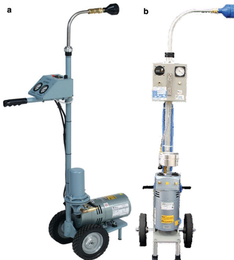
Fig. 6.13 Portable air samplers with the “goose neck” design. a Courtesy of the HI-Q company www.hi-q.net . b Courtesy of F&J Specialty Products, Inc.; www.fjspecialty.com )
