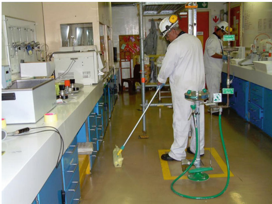
Fig. 6.5 An RP technician performing a contamination survey using a masslinn mop to obtain a large area swipe (Courtesy of ESKOM and Koeberg Radiation Protection Department)
