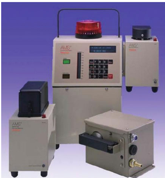
Fig. 11.22 Depicts the AMS-4 unit with the optional inline module (Courtesy of Thermo Fisher Scientific, www.thermofisher.com )
