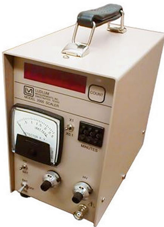
Fig. 11.15 The Ludlum Model 2000 scaler commonly used as a bench-top counting station (Courtesy of Ludlum Measurements, Inc. www.ludlums.com )
