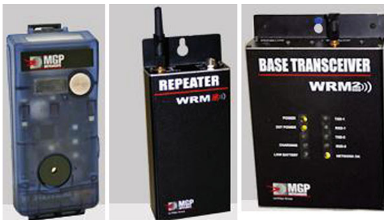
Fig. 10.8 The Mirion Technologies wireless remote monitoring system consisting of, from left to right, the WRM2 transmitter unit, the WRM2 repeater unit, and the WRM2 base station transceiver (Courtesy of Mirion Technologies, www.mirion.com )
