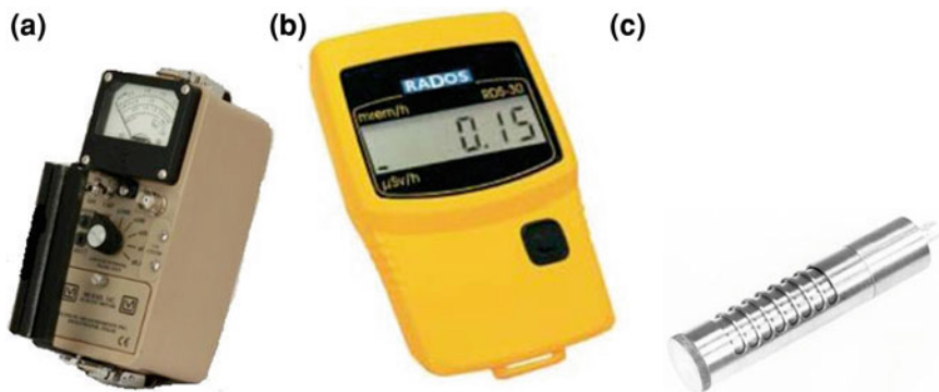
Fig. 11.3 a Ludlum Model 14C G–M survey meter. c Ludlum Model 44-6 G–M probe (Courtesy of Ludlum Measurements, Inc. www.ludlums.com ). b Mirion Technologies RDS-30 G–M dose rate meter (Courtesy of Mirion Technologies www.mirion.com )
