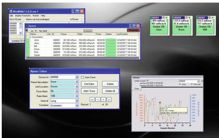
Fig. 10.7 Computer screen depicting the various parameters displayed by a teledosimetry base station (Courtesy of Mirion Technologies, www.mirion.com )
