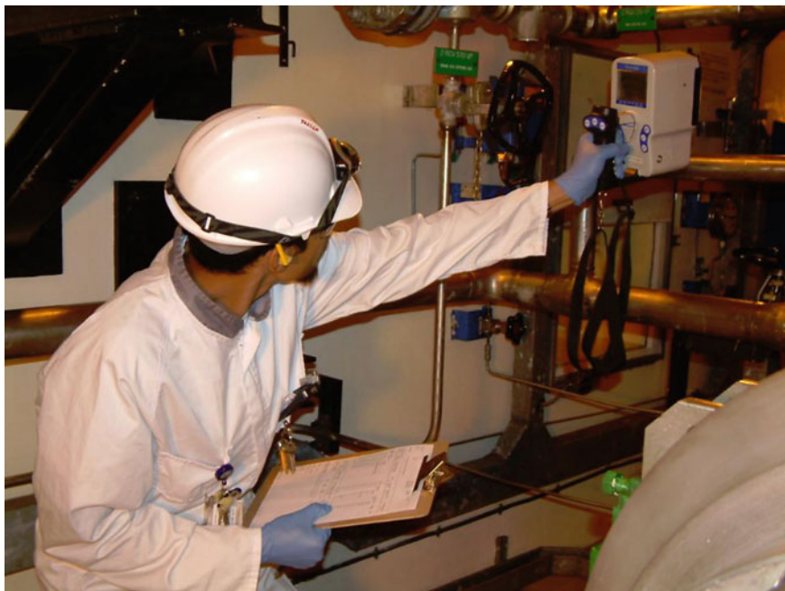
Fig. 6.2 A radiation protection technician performing a radiation survey in the field (Courtesy of ESKOM and Koeberg Radiation Protection Department)
