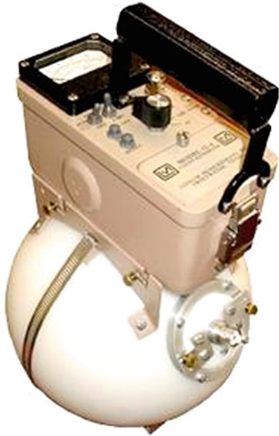
Fig. 11.6 The Ludlum Model 12-4 neutron dose rate survey instrument (Courtesy of Ludlum Measurements, Inc. www.ludlums.com )
