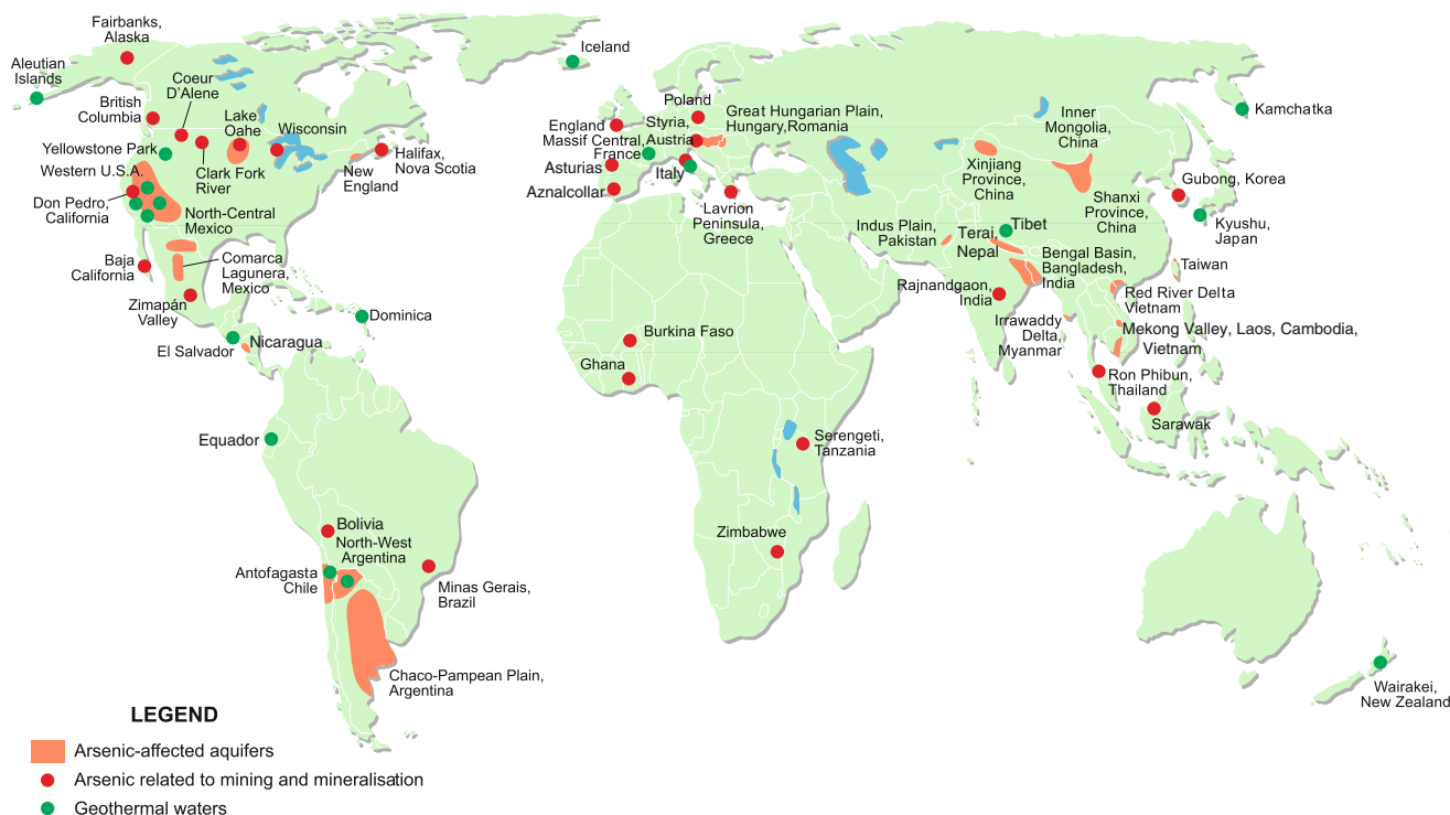
Fig. 12.2 Occurrence of documented arsenic problems in groundwater (arsenic >50 \mu\text{g L}^{-1} ) in major aquifers and environmental problems related to mining and geothermal sources
