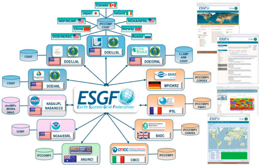
Fig. 7.6 Federation of ESGF showing collaborations between a few of its remote data centers, data archives, and potential data transfers between sites. For example, the U.S. DOE/LLNL portal (at the top) harvests IPCC/CMIP5 data from 10 countries. That is, the original data resides at the data centers, but subsets of the data are replicated at LLNL for backup, better access and use. The DOE/LLNL portal URL is http://pcmdi9.llnl.gov
