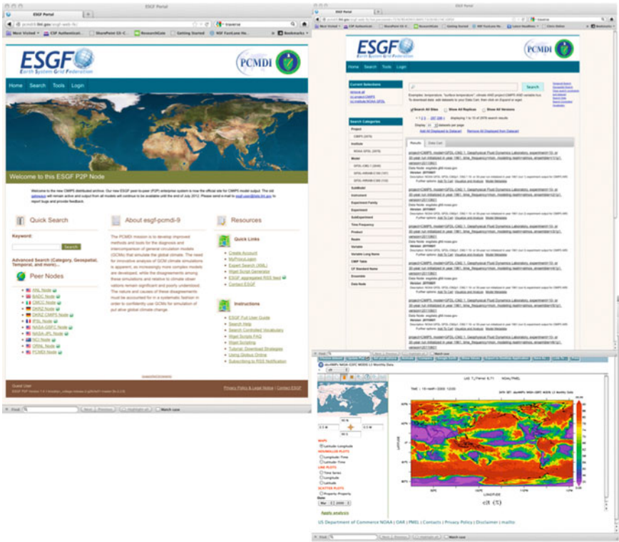
Fig. 7.4 The ESGF node installation script deploys the home page of a minimally configured web front-end application, as shown to the left . Included on the home page are search capabilities, information pertaining to the node and organization, quick links to commonly used tools, links to other ESGF nodes, and analysis tools. Example search page and analysis/visualization results are shown on the right
