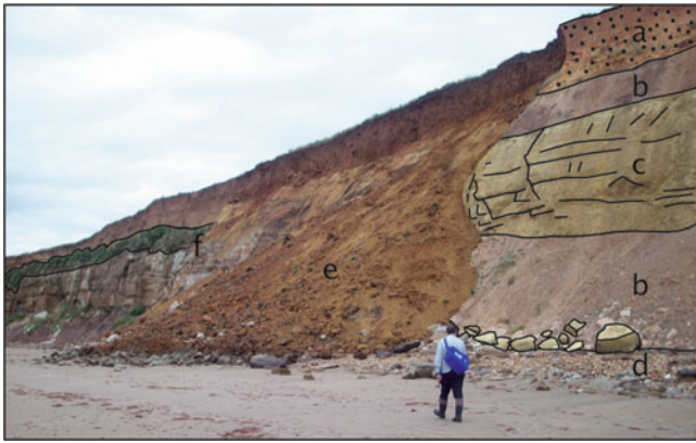
Fig. 5 Rockfall from the Sudmoor Sandstone between Sudmoor Point and Chilton Chine: (a) Quaternary sands and gravels, (b) Wessex Fm. mudstones, (c) Wessex Fm. sandstones (Sudmoor Sandstone), (d) large boulders of sandstone, (e) rockfall debris, (f) vegetation indicating excessive seepage
