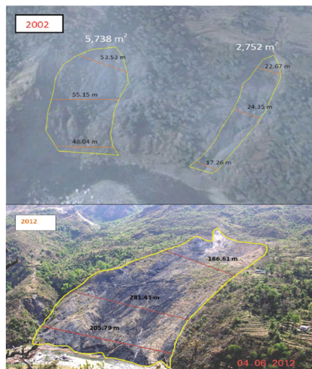
Fig. 4 Google snapshot of year 2002 and field photograph of 2012 to show the dynamic nature of the landslide
