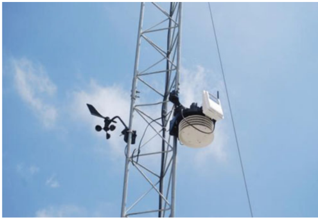
Fig. 9 Meteorological station located on the monitoring site. Rainfall is monitored at 5 min intervals
