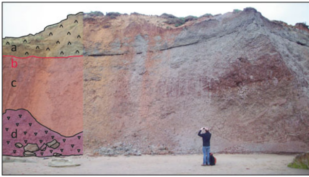
Fig. 3 Persistent and active shear surface underlying the Roughlands Landslide. (a) colluvium, (b) shear surface, (c) in situ varicoloured mottled mudstones, (d) accumulated talus cone of colluvium
