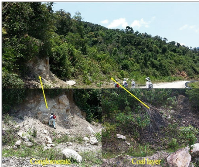
Fig. 8 Coal layer and fractured rock consisting of sandstone, mudstone and conglomerate on landslide No. 18
