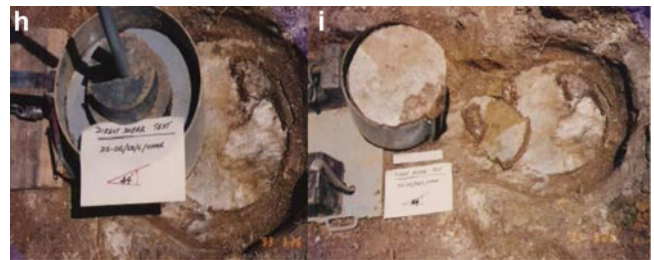
Fig. 5 Observation of uniformity of plane of failure (h and i) after the test (Note: The visual characteristics of slip surface and the past movement history of landslide provide an ample evidence of residual conditions)
