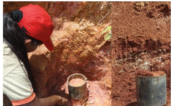
Fig. 4 Intact soil was obtained by high quality manual sampling method; Zone 1; Nuwara Eliya District
