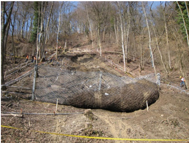
Fig. 4 Experimental landslide triggered by irrigation in the framework of the research project TRAMM (Springman et al. 2012). A comprehensive set of measurements provided insight into the wetting of the soil as well as precursors and movements prior to the release
