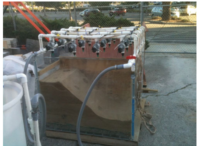
Fig. 1 Plexiglas container, slope made of double washed sand at a 30° inclination, and the rain simulator used in this study
