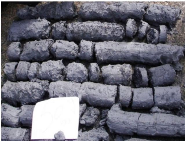
Fig. 2 Slip zone of Suoertou landslide from borehole ZK3
