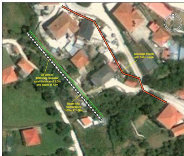
Fig. 18 Satellite image of the studied area, showing the proposed retaining wall and drainage trench, for the protection of the houses above the landslide
