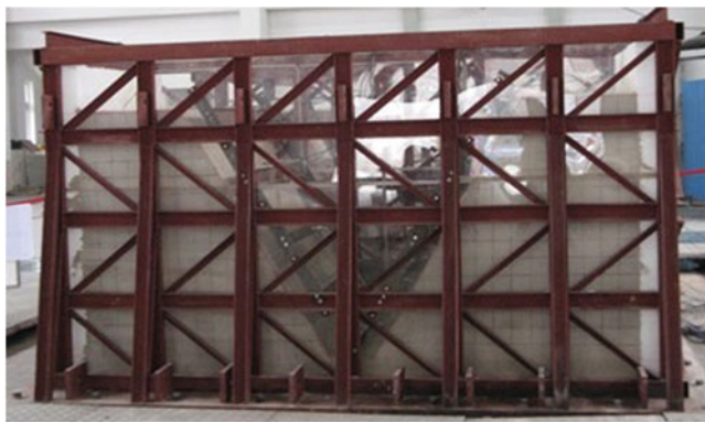
Fig. 3 The slope model 1 before the test (the left part is the limestone slope and the right part is the mudstone slope)
