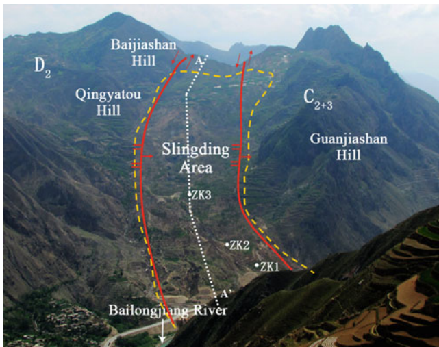
Fig. 1 Overview of the Xieliupo landslide and locations of boreholes (ZK1-ZK3) on the landslide
