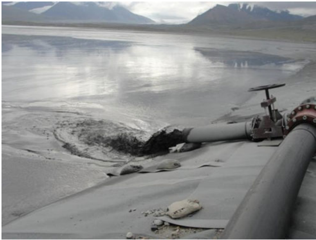
Fig. 1 July 2012. Tailings pit. Discharge of pulp (sludge) from the mineral separation plant at the Kumtor mine
