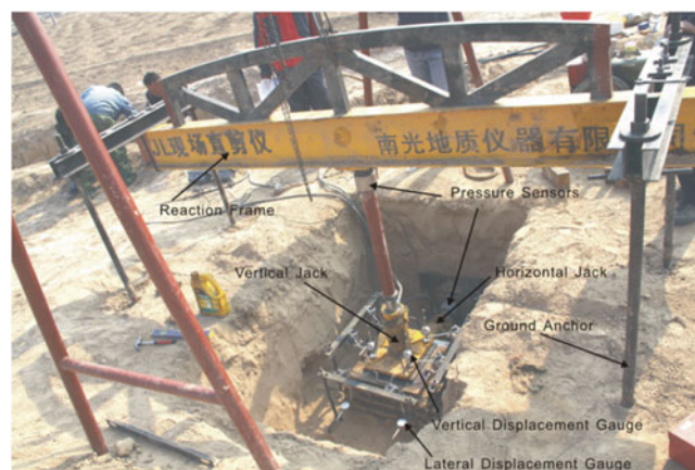
Fig. 1 Conventional in-situ large scale shear test apparatus
