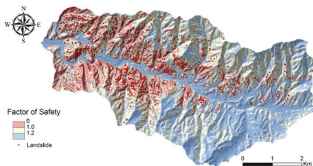
Fig. 4 Factor of safety evaluated using rainfall intensity of rainstorm after 8 h
