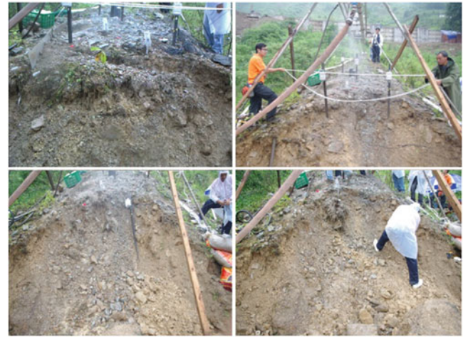
Fig. 9 The final shape of scarp and slope after failures, demonstrating progressive failure during the test
