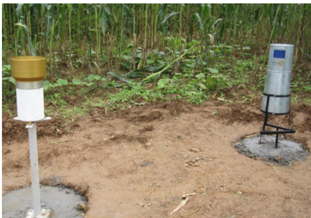
Fig. 4 Automatic rain gauge (on the left), Tipping Bucket, and manual rain gauge (on the right), standard rain gauge installed in the project site for rainfall observation
