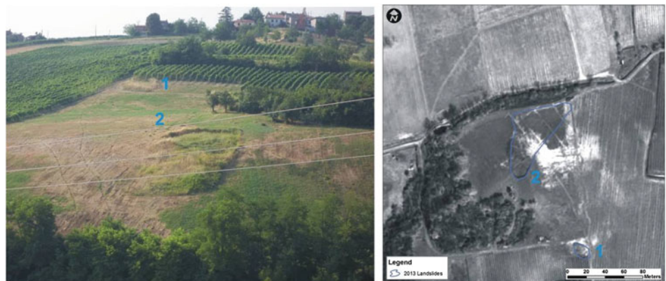
Fig. 5 Examples of shallow translational landslides triggered in uncultivated field detected through field work and Pleiades images
