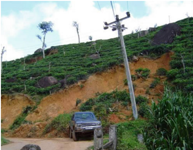
Fig. 9 An observation of relatively circular modes of failure in colluvium formation
