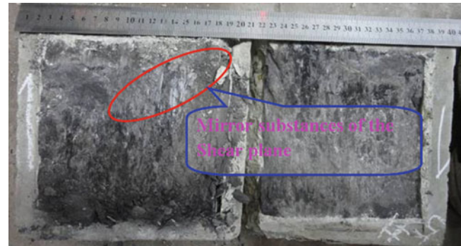
Fig. 2 Destruction of the samples and the observed slickensides
