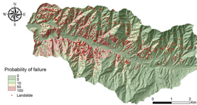
Fig. 2 Probability of failure evaluated using rainfall intensity of rainstorm after 8 h
