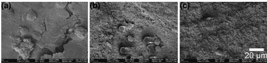
Fig. 8 SEM pictures of a cell layer grown on modified carrier surfaces: a cell layer on the rough and inhomogeneous carrier as received, b cell layer on the smooth carrier polished using plain paper, c cell layer on the structured carrier polished using polymer sheet (adapted from Wiegandt et al. [60])
