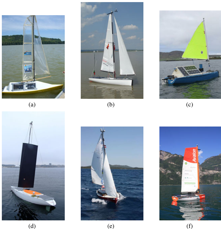
Fig. 8 Autonomous sailing vessels with a length of more than 2 m: (a) IBoat, ISAE (b) FASt, University of Porto (c) Pinta, University of Aberystwyth (d) Beagle-B, University of Aberystwyth (e) ASV Roboat, INNOC (f) Avalon, ETH Zurich
