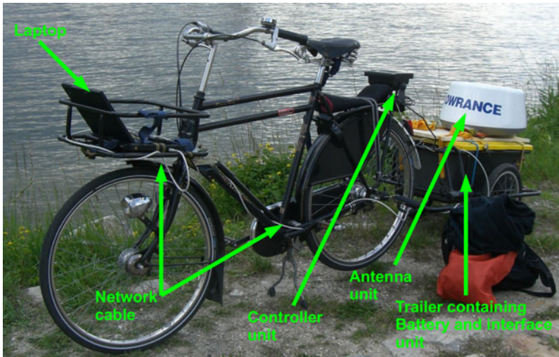
Fig. 5 The sample data acquisition setup
