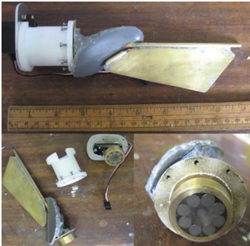
Fig. 5 The rudder assembly, magnetic linkage and servo
