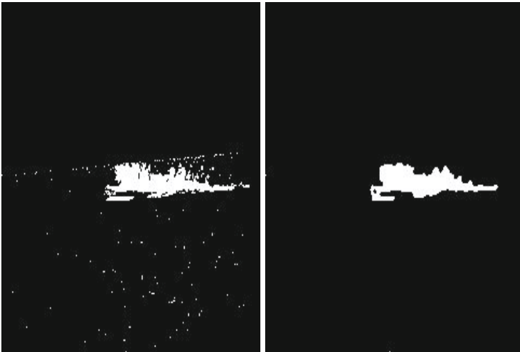
Fig. 4 Morphologic Cleaning: The left side shows the image after detecting the sea pattern and the right side shows the image after applying the morphologic methods: Cleaning and Fill filter
