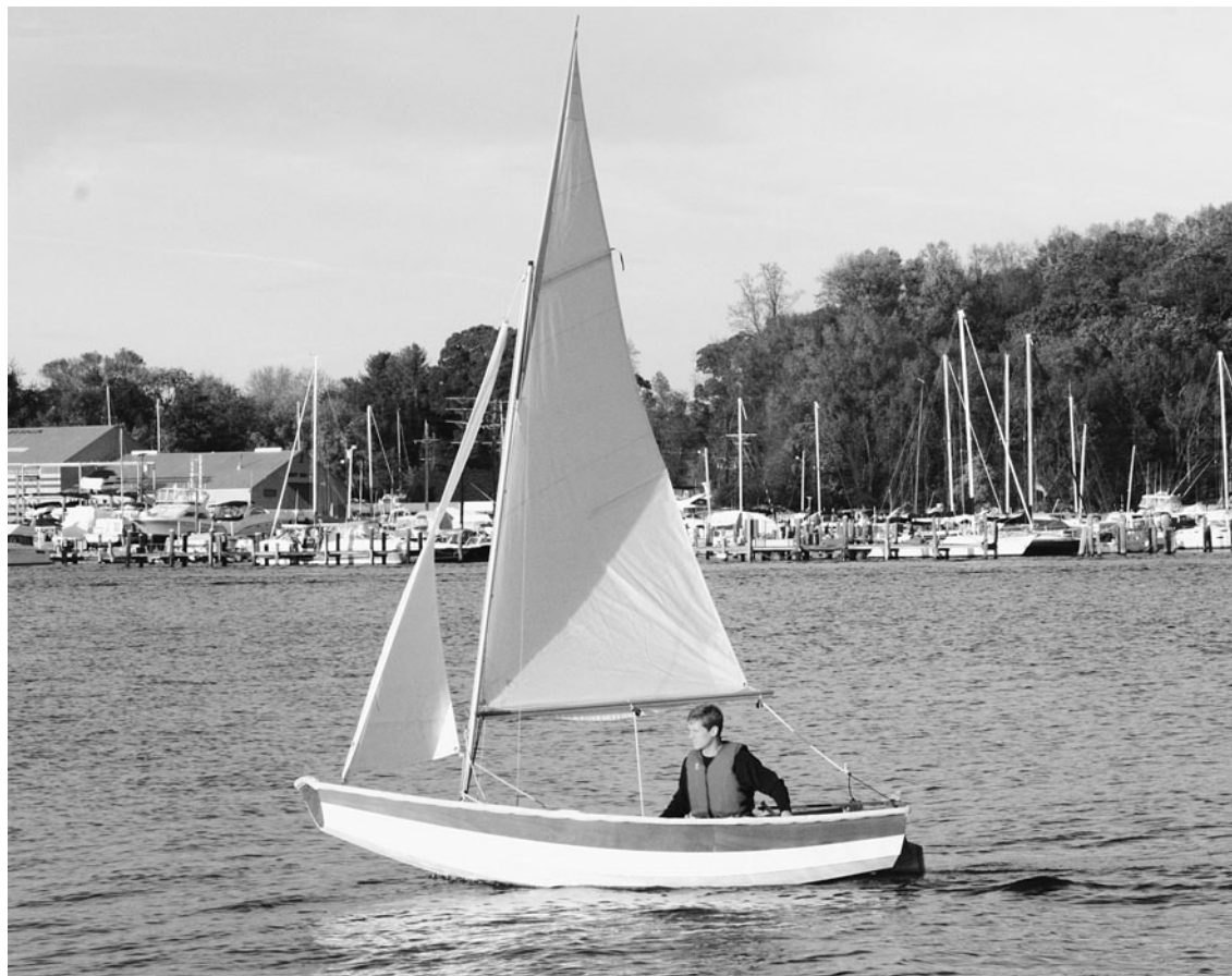
The sliding-gunter rig provides performance when sailing to windward, but still offers the advantages of a gaff. (Chesapeake Light Craft)
