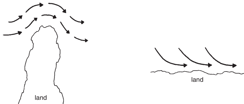
The land can influence wind direction in a number of ways. For example, a breeze will bend around a headland (left), and a wind nearly parallel to the land will often become even more parallel.
