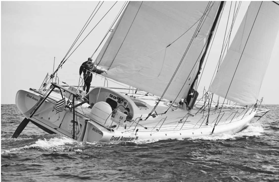
An Open 60 has a broad, shallow hull optimized for sailing downwind. (Billy Black)
