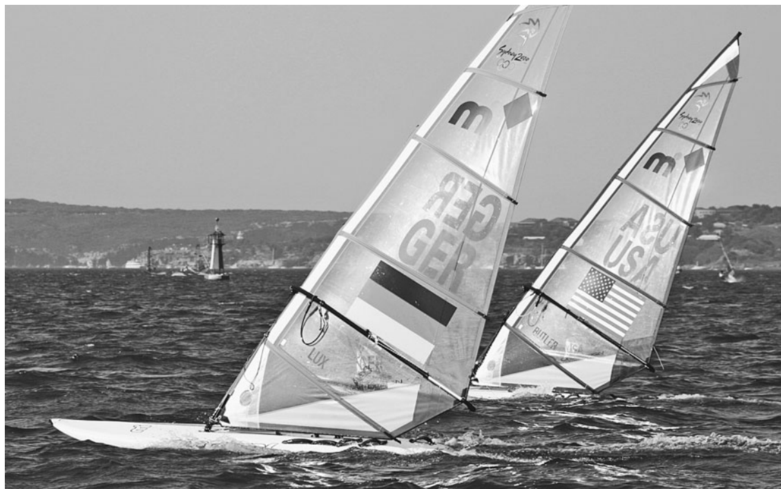
A windsurfer shifts his weight and position along the boom to alter the CE and CLR of the boat. (Daniel Forster)
