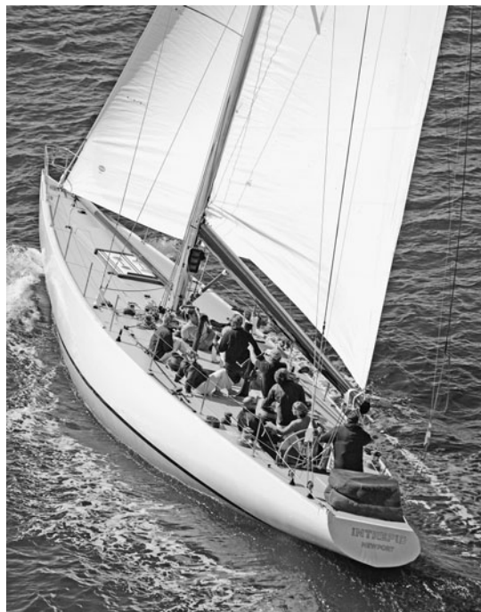
A 12-meter yacht employs a narrow hull shape optimized for sailing to windward. (Billy Black)
