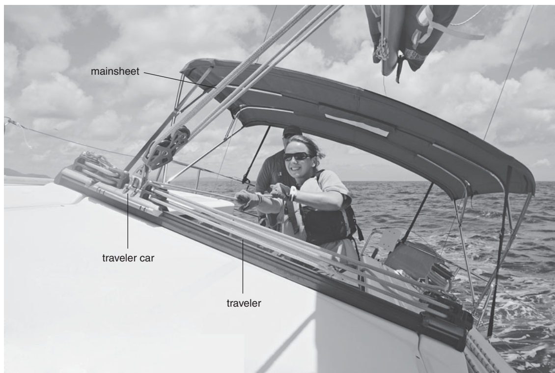
When sailing to windward on racing boats and performance cruisers, the mainsheet is regarded primarily as a device for controlling twist, and the main traveler is used to control angle of attack. (Erik Skallerup and Domenic Mosqueira/YachtShots, BVI)
