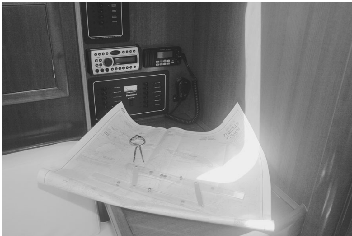
The tools of the navigator include parallel rules that allow you to “walk” your course to a nearby compass rose, and dividers, which are used to measure distances. (Erik Skallerup and Domenic Mosqueira/YachtShots, BVI)
