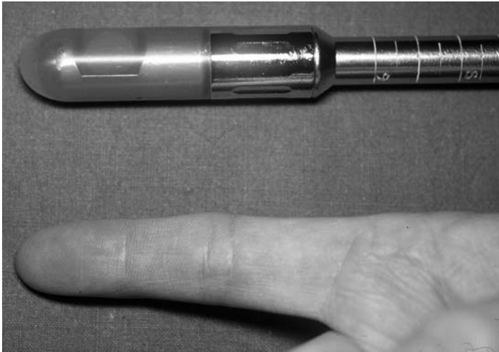
FIGURE 11.14. The transducer protected by a plastic cone.
