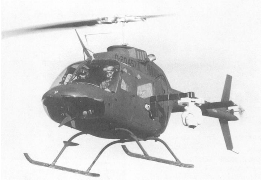
FIG. 38—Conducting an airborne infrared roof moisture survey from a helicopter.
