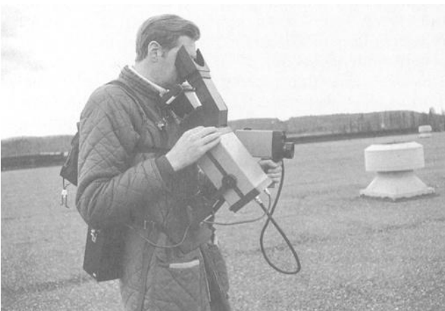
FIG. 36—Surveying a roof with an infrared scanner.
