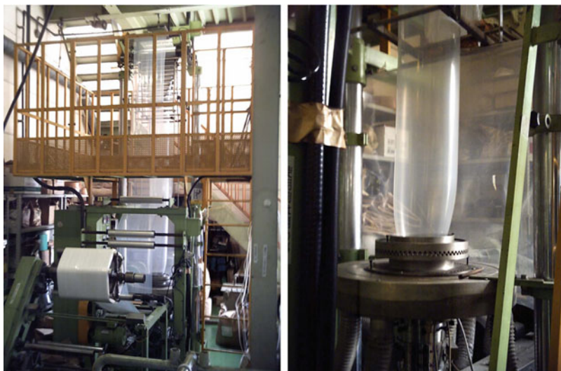
Fig. 16 Blown film processing of Bionolle
