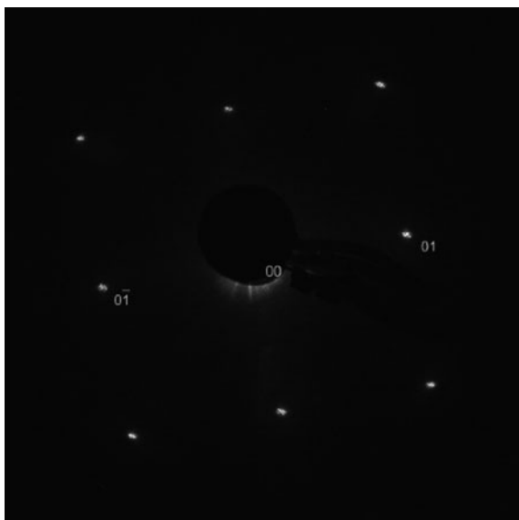
Fig. 4.2 LEED pattern of a clean Ni(100) acquired using a 103 eV electron beam energy [5, 6]
