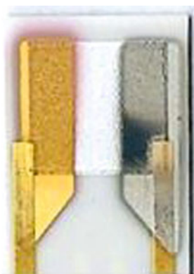
Fig. 7 Electrode degradation during sensor ageing: carbon deposition on platinum electrode
