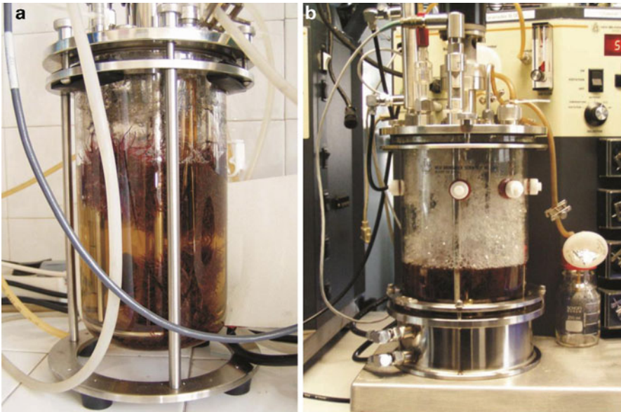
Fig. 11.4 14-days-old B. vulgaris cv. Detroit Dark Red hairy roots cultivated in stirred tank bioreactors: clump formation between the electrodes in 3-L vessel (a); homogenous culture during fed-batch cultivation in 5-L vessel (b)
