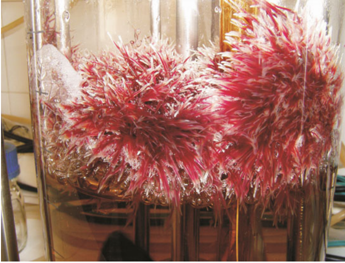
Fig. 11.1 Self-immobilization of 14-days-old B. vulgaris cv. Detroit Dark Red hairy roots on the medium surface during cultivation in stirred tank bioreactor
