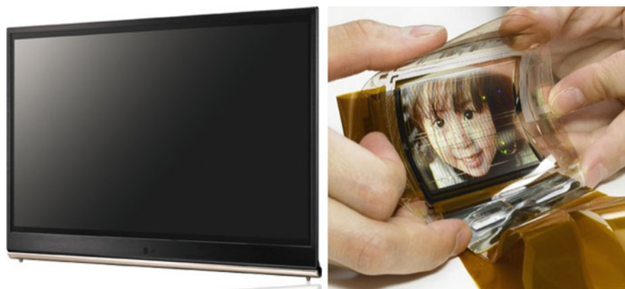
Fig. 1.3 Left A wide range of electronic devices that use organic semiconductors are already being commercialized by technological corporations, like this LG@15EL9500 television with OLED technology. Copyright LG. Taken from [32]. Right Flexible organic display of 2.5 inch, 160 \times 120 pixels manufactured by Sony®. It is able to reproduce 16.7 million colors (24 bits). Copyright Sony (2007). Taken from [33] (Color figure online)
