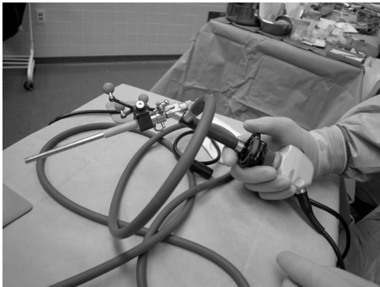
Fig. 1. An endoscope. Three spheres arranged in a triangle are used by the neuronavigator to determine the position of the endoscope relative to the patient
