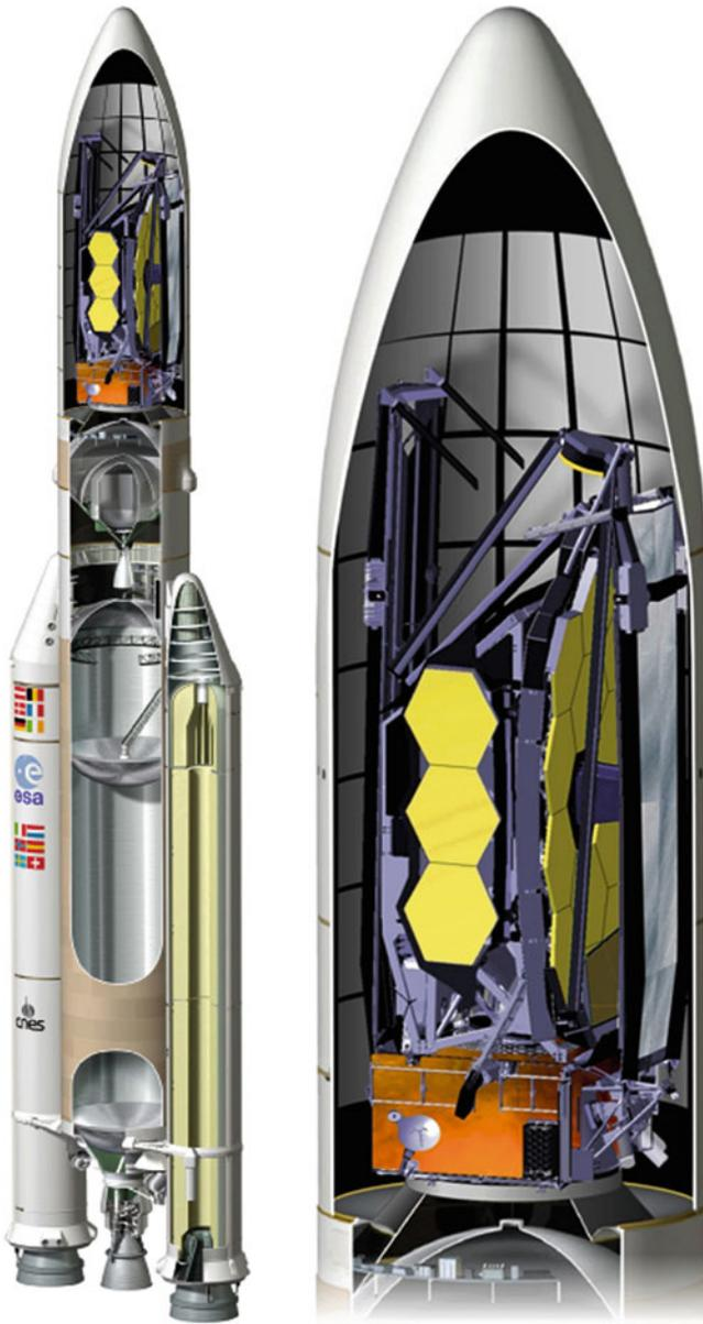
**FIG. 12.6** The Ariane 5 rocket pictured above will launch JWST into space. The main telescope mirror will measure 6.5 m in diameter, too large to launch in one piece. It will consist of 18 individual mirror segments mounted on a frame which will be folded inside the the Ariane 5 at launch. The *right panel* shows the a closeup of JWST stowed inside the Ariane 5 (Credit: Arianespace – ESA – NASA)
