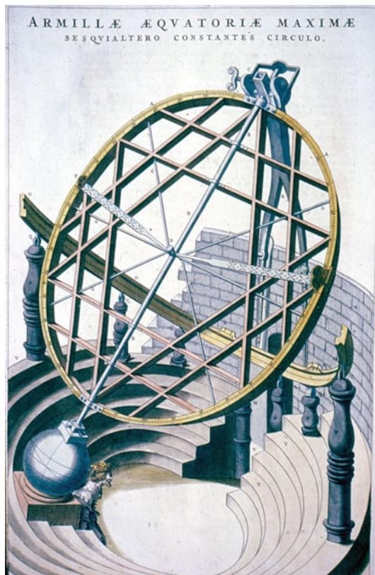
**FIG. 1.2** One of the sophisticated instruments that Tycho used to make his measurements. This instrument was used to measure the angular position of stars above or below the celestial equator. The *large circle* has a diameter of 2.7 m. This instrument was completed in 1585 (Published in 1662 and based on Tycho's original version, this illustration is by Willem Blaeu, a former assistant at Tycho's Hven observatory. Credit: Collection of Owen Gingerich)
