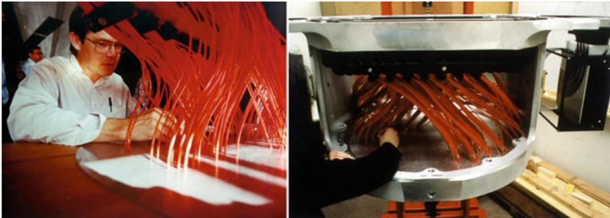
**FIG. 5.2** The plugboard for the Sloan Digital Sky Survey fiber spectrograph. A thin plate of metal is mounted on the back of the telescope. This plate has a set of about 500 holes drilled into it at exactly the locations of 500 galaxies in the direction that the telescope is pointing. Each hole is plugged with an optical fiber, which carries the light from one galaxy down to a big spectrograph. In this way 500 galaxies can be observed at once (Credit: Fermilab Visual Media Services)
