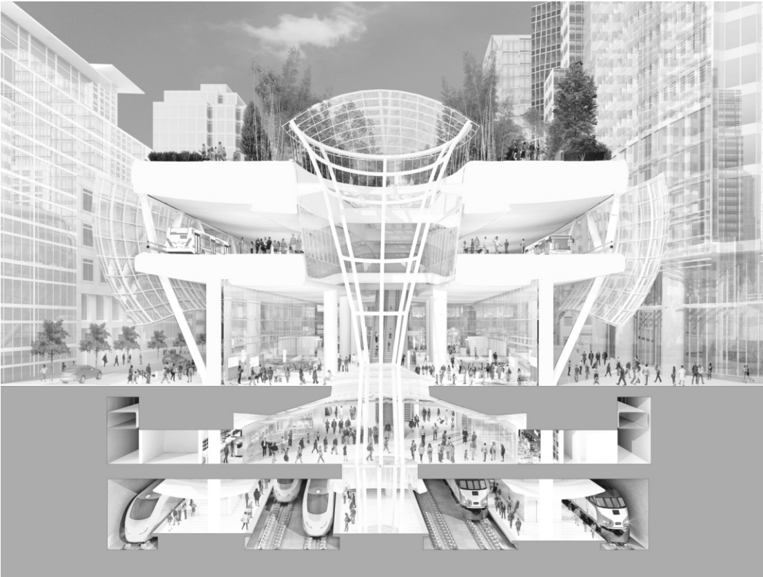
Figure 2-2. Cross-section rendering, Transbay Transit Center, San Francisco, California. (Project Architect: Pelli Clarke Pelli. Renderings courtesy of the Transbay Joint Power Authority.)
