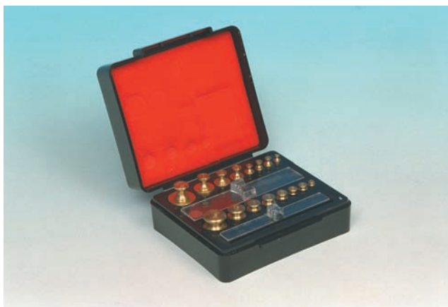
FIGURE 14-2 Pharmaceutical weights should be corrosion-resistant and handled with forceps.
