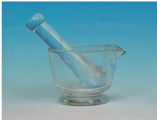
FIGURE 14-4 A glass mortar and pestle is preferable for mixing liquids and semisoft dosage forms.
