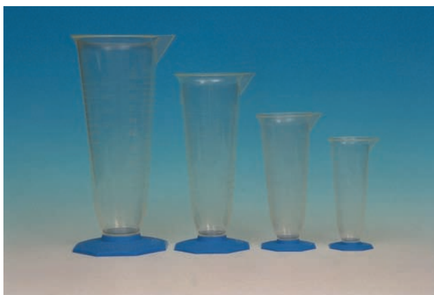
FIGURE 14-6 Conical graduates have a wide mouth and a narrow base.
