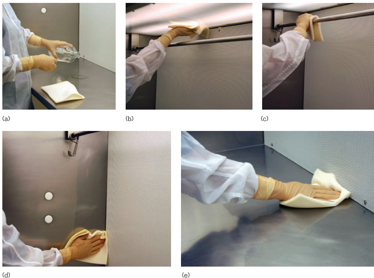
FIGURE 15-8a-e Preparation of a horizontal laminar flow workbench (HLFW) (Courtesy of the University of Tennessee Parenteral Medications Lab).
