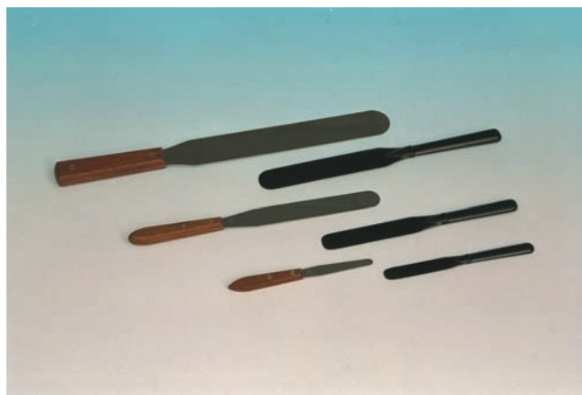
FIGURE 14-3 Spatulas, available in stainless steel and hard rubber or plastic, are used to transfer solid ingredients to weighing pans.
