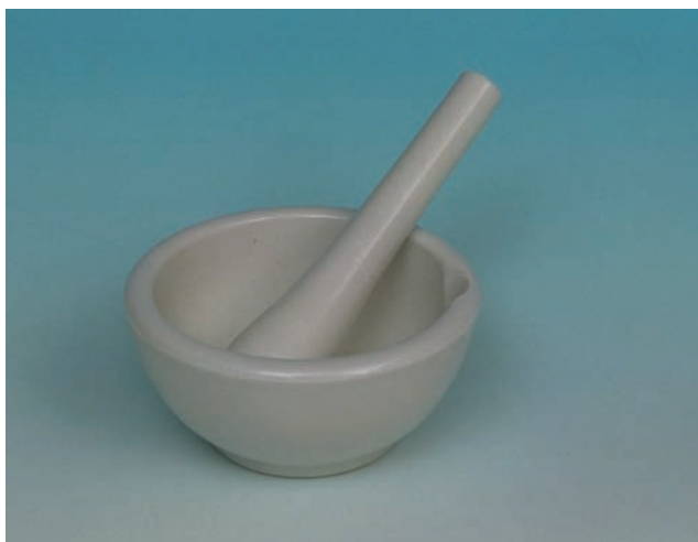
FIGURE 14-5 A porcelain mortar and pestle is used for trituration of crystals and large particles.
