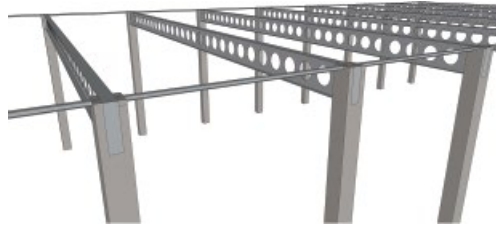
Figure 6.68 Typical single-storey building with cellular beams.
