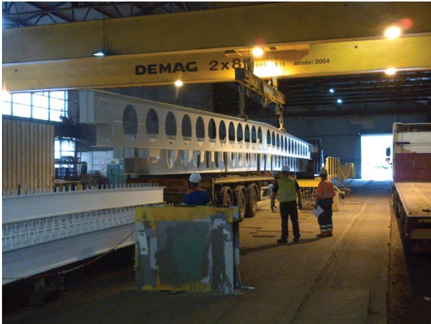
Figure 3.17 Loading of a cellular beam – here a roof girder in industrial building. Cellular beams are also solutions with minimal floor depth for multistorey framed buildings. © ArcelorMittal.
