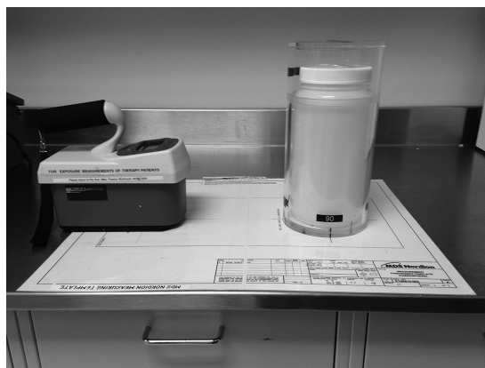
Figure 7.15 Setup for TheraSphere posttreatment ion chamber survey meter exposure rate reading of residual activity, using the fixed-geometry template provided by the manufacturer (30-cm waste jar center-to-ion chamber center distance). The average of four readings, with the waste jar plus shield rotated 90^\circ between each, is compared with that from the v-vial in shield prior to treatment, to estimate the fraction of total v-vial activity delivered to the patient.
