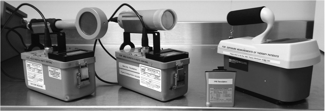
Figure 7.10 Radiation detectors employed during ^{90}\text{Y} microspheres radioembolization. From left to right: pancake probe G-M survey meter (protective cover removed for detecting \beta particles); \beta probe survey meter with plastic attenuator (for measuring count rate from TheraSphere microspheres at the output line-microcatheter junction); electronic personal dosimeter (for measuring the external bremsstrahlung dose rate from the TheraSphere vial); and ion chamber survey meter (for measuring external bremsstrahlung exposure rate from the patient's liver containing microspheres).
