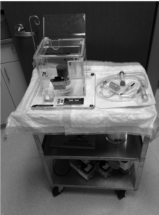
Figure 7.11 TheraSphere treatment delivery cart. Top shelf: dose vial in acrylic shield and lead pot, inside the infusion delivery box, and dose administration kit. Middle shelf: biohazard bag for collecting potentially radioactive garments and surface coverings, and a 2-L Nalgene waste jar inside its shield. Bottom shelf: \beta scintillator, pancake G-M, and ion chamber survey meters.
