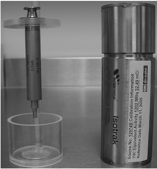
Figure 7.2 NIST-traceable ^{90}\text{Sr}/^{90}\text{Y} transfer standard for calibration of dose calibrators for assaying ^{90}\text{Y} Zevalin ( 2\sigma = 4.7\% ) that simulates 4 mL of ^{90}\text{Y} Zevalin in a 10 mL Becton–Dickinson plastic syringe. The standard is accompanied by a table of correction factors for other solution volumes that vary linearly from 0.983 at 9 mL to 1.017 at 1 mL.
