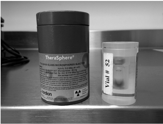
Figure 7.6 TheraSphere patient dose delivery v-vial in its acrylic shield and associated lead pot.
