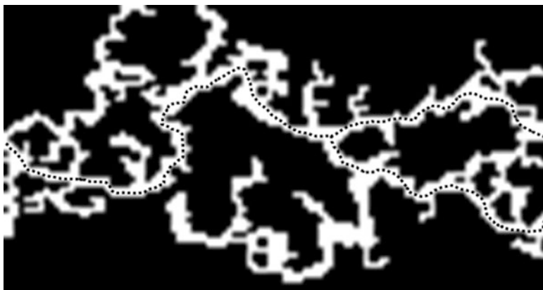
Fig. 2.23 Schematic illustration of the trapping effect on a random walker in a ramified pore space (white). The dotted lines represent two possible trajectories of the random walker across the pore space cluster. If the random walker gets temporarily “trapped” in a dead end or in a side area badly interconnected to the main cluster, it will take a long time until the main transport pathways across the cluster will be rejoined
