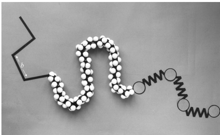
Fig. 5.5 Different versions of model chains for polymers. Middle section : Space-filling atom model of polyethylene. The hydrogen atoms are represented in white as hemispheres with a radius equal to the van der Waals radius. This is the radius that would determine nearest atom distances in crystalline structures. Left : Freely jointed model chain. Right : Bead-and-spring polymer model. (Reproduced from Ref. [14] with kind permission of © Elsevier 1988)
