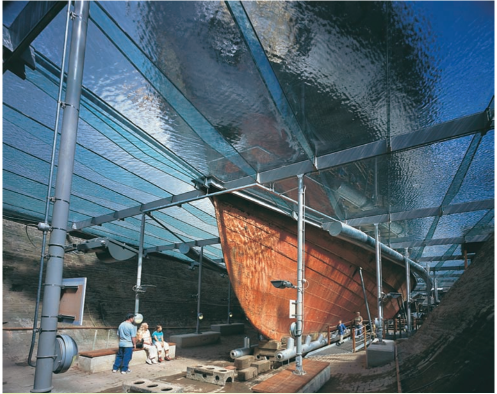
Figure CS2.2 The underside of the ship, showing the glass plates sealing the hull from exposure to the elements.
