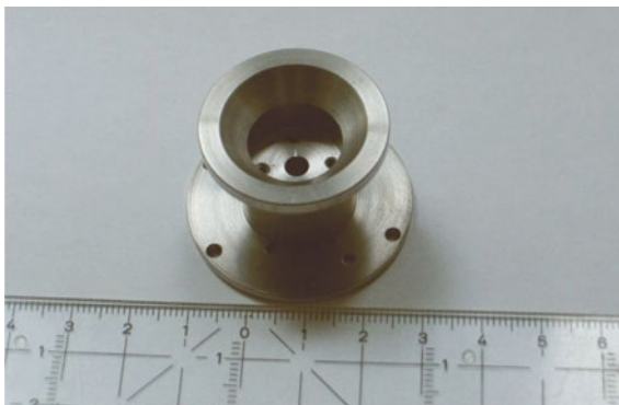
Fig. A.1 The heart of the old furnace. The sample holder is mounted inside, the heating wire is coiled outside
