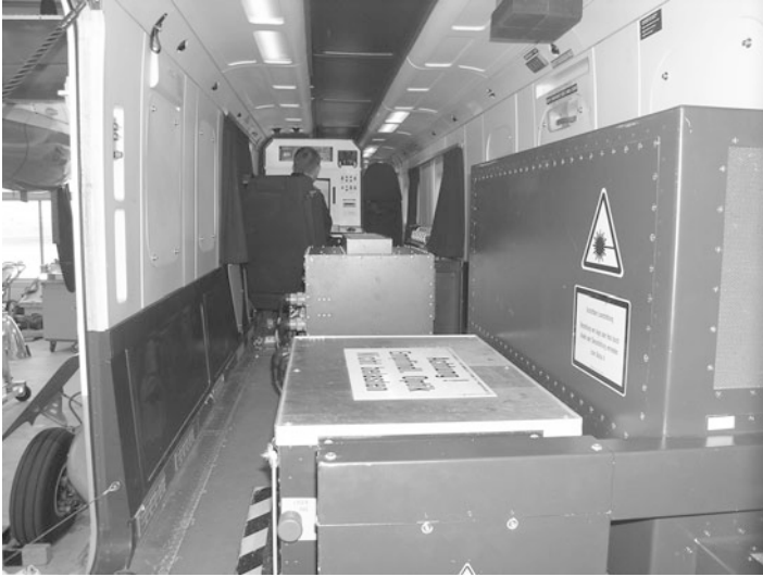
Fig. 3 View of the interior of the Do228 57+04. All sensors are controlled by an operator from the central computer console (© BfG, CCME)
