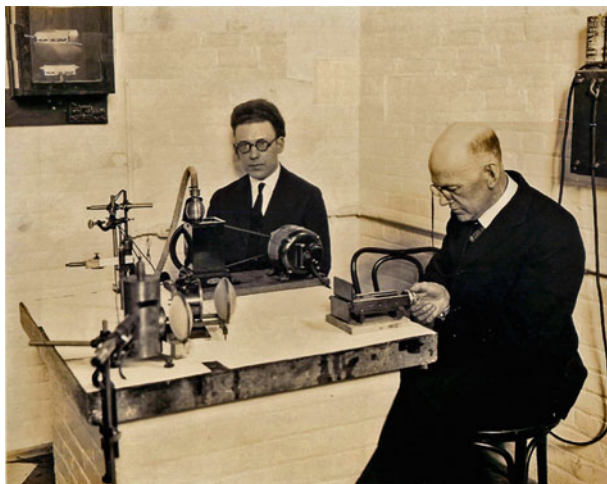
Fig. 1.7 Nichols and Tear in a laboratory of the National Electric Light Association in Cleveland, Ohio, where Nichols was the Director. The Hertzian type oscillator is within the metal container on the left. The output is collimated by a paraffin wax lens onto a Boltzmann interferometer which Nichols is adjusting. The reflected beam is then focused by the second lens onto a radiometer detector (for details of the experimental setup see [19], photograph courtesy of J. D. Tear’s relatives)
