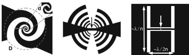
Fig. 3.25 Layout of three planar antennas. From left to right: logarithmic-spiral, logarithmic-periodic, and double-slot antenna. The metallized parts are shown in black. The arrows indicate the positions of the detecting or emitting element. Some typical dimensions are given (for explanation see text)
