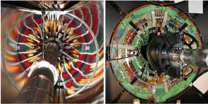
Fig. 8.15 View of the BPIX detector in its final position. Left The picture shows the BPIX detector inside CMS enclosing the central beam pipe. The camera is placed inside the detector supply tube and the detector endflange covered by the cooling lines and signal and power cables can be seen. Right Picture of the connection area PP0 at the far end of the pixel volume. The connection of power cables ( green cables ), optical fibers (wrapped in red rubber bands ) and cooling lines are visible. In the foreground the beam pipe suspension is shown
