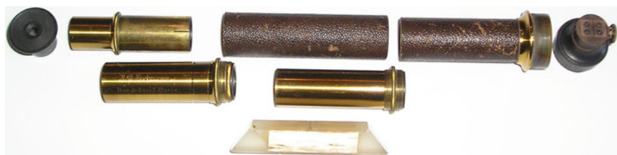
Fig. 3.3 Janssen's direct-vision spectroscope as constructed by J.G. Hofmann. © Author's collection
