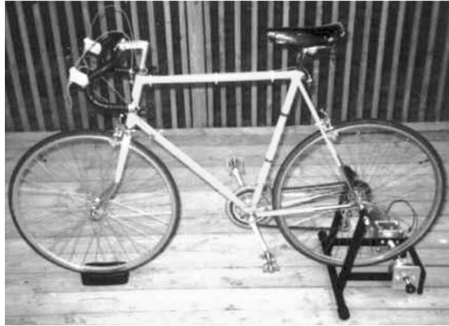
Figure 8.1 Exercise bicycle with magnetoalternator to generate electrical energy during workouts at Duke University.
