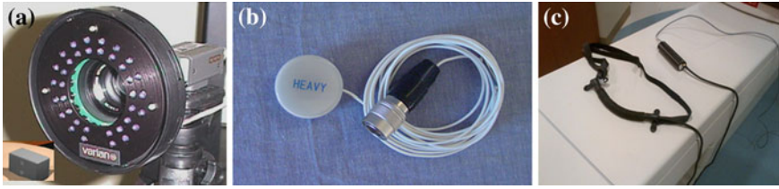
Fig. 2.9 Respiratory monitoring devices used in 4D CT. (a) Two reflective markers on a plastic box and an infrared camera from Varian; (b) A pressure sensor from Anzai; and (c) Air bellow and pressure sensor from Philips
