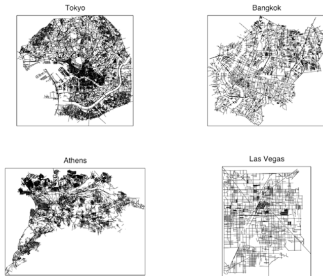
■ 'Axial maps' of cities, in which straight lines designating open spaces are extended until they cross, reveal distinct classes of urban structures, as shown here in examples of open (Tokyo, Bangkok), dense (Athens), and intermediate (Las Vegas) structures. (Credit: from R. Carvalho & A. Penn, Physica A 32 , 539–547 (2004).)
