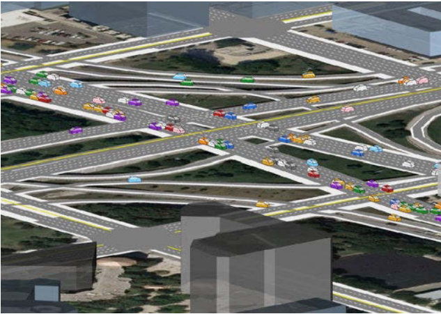
■ Traffic models suppose that vehicles move along predefined highways according to simple rules, chosen largely to avoid collisions. (Credit: Courtesy of Argonne National Laboratory - Transportation Research and Analysis Computing Center.)
