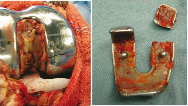
FIGURE 1-2. (A and B) A fractured femoral component.
