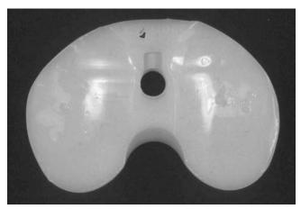
**FIGURE 2-2.** Three-year retrieval of a failed Hylamer-M tibial plateau demonstrating an unexpectedly high wear rate with corresponding wear and debris-induced inflammatory tissue response.
