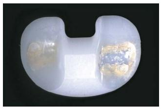
**FIGURE 22-2.** Retrieved polyethylene liner (treated by gamma irradiation in air) demonstrating surface delamination (mode 1 wear).
