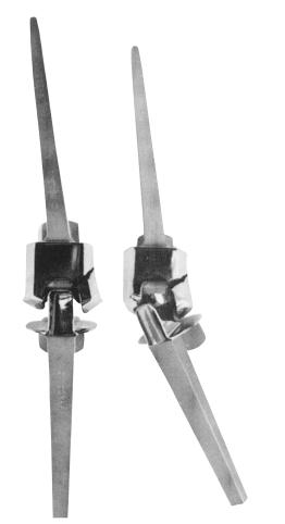
**Figure 20-6.** The Herbert total knee arthroplasty prosthesis. Pictured are prosthetic medial condylar fractures that resulted in the prosthesis being pulled from market soon after its release. (From Murray, Wilde, Werner,<sup>21</sup> by permission of *J Bone Joint Surg Am.*)
