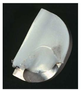
**FIGURE 19-6.** Metal-backed tibial component with wear through of the peripheral polyethylene in a pattern similar to anteromedial wear in an osteoarthritic varus knee.
