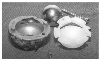
**FIGURE 2-20.** A 1-year conventional UHMWPE, primary acetabular liner demonstrating crack initiation and propagation. Failure initiated at a sharp edge of a locking point. (From Tradonsky, Postak, Froimson<sup>129</sup> by permission of *Clin Orthop.*)
