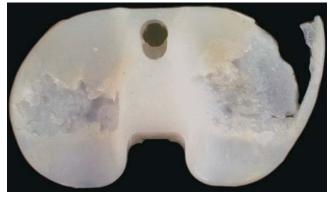
**FIGURE 2-3.** Six-year retrieval of a heat-pressed tibial component associated with polyethylene fatigue and early delamination.
