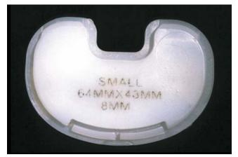
**FIGURE 22-3.** Undersurface of retrieved liner demonstrating minimal backside (mode 4) wear.
