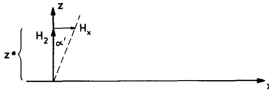
Figure 12.13 Longitudinal component H_x of the field for E_y of Fig. 12.12.
