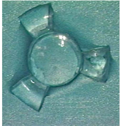
Fig. 13.7. Flexible, foldable lens prototype
