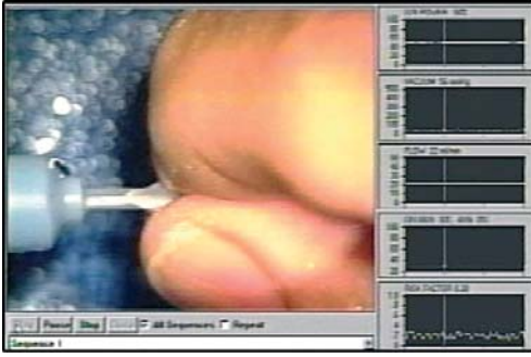
Fig. 24.4. Phacoemulsification tip in sonic mode being grasped with an ungloved hand, demonstrating lack of heat generation
