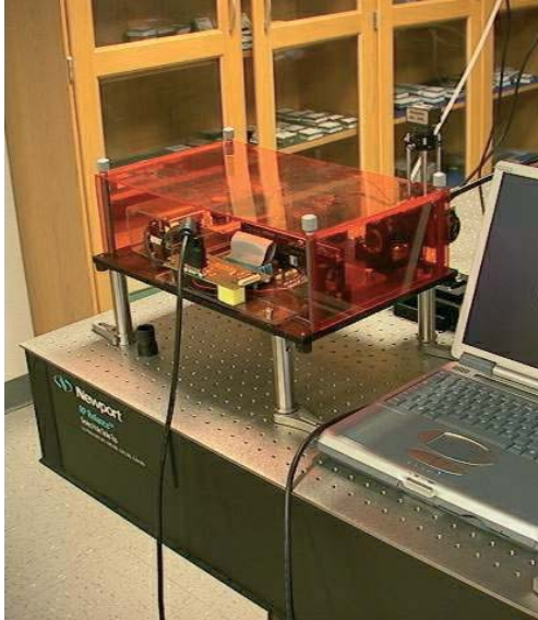
Fig. 17.11. Digital light delivery device (DLDD). (Courtesy of Calhoun Vision Inc.)
