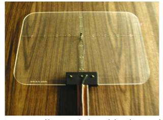
**FIGURE 6.10.** Maddox cross with a fixation light in the center. The scale of the cross is adjusted so that when the patient is at 50 cm, the engraved numbers on the plastic panel indicate the amount of deviation in degrees.
