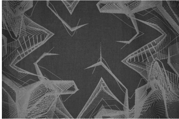
Fig. 3.2 Laser engraving on rayon/polyester blended fabric
