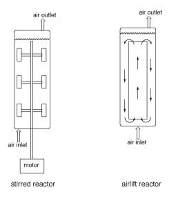
Figure 3 Schematic of stirred and airlift bioreactors
