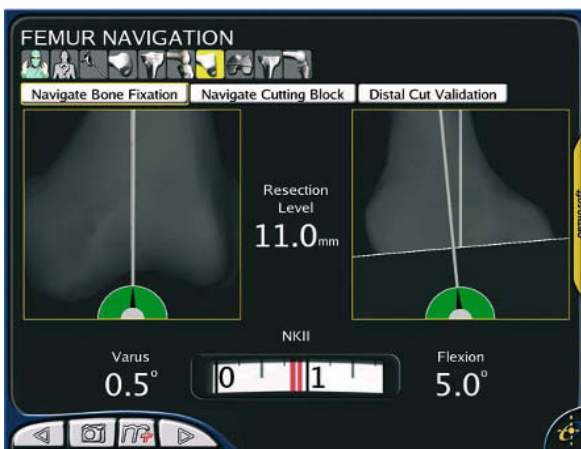
■ Fig. 21.5. Distal femoral resection, varus-valgus position and flexion can all be visualized in a easy to read screenshot with the current software
