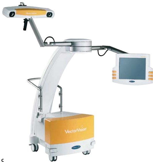
Fig 74.1a–c. Intra-operative 3D imaging using a fluoroscope (Siemens ISO C-3D) with the patient placed on a carbon fiber table (a) and transferring the dataset via NaviLink (b) to the BrainLab VV 2 system (c)
