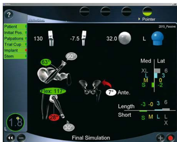
■ Fig. 48.4. Screen display after registration of the stem position. The simulation allows modification of antetorsion and CCD angle by choosing different modular necks and leg length and offset by the ball size and neck length
