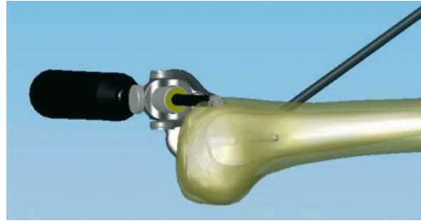
■ Fig. 16.11. Computer aided design model of the Praxiteles milling robot, shown milling the anterior femoral plane
