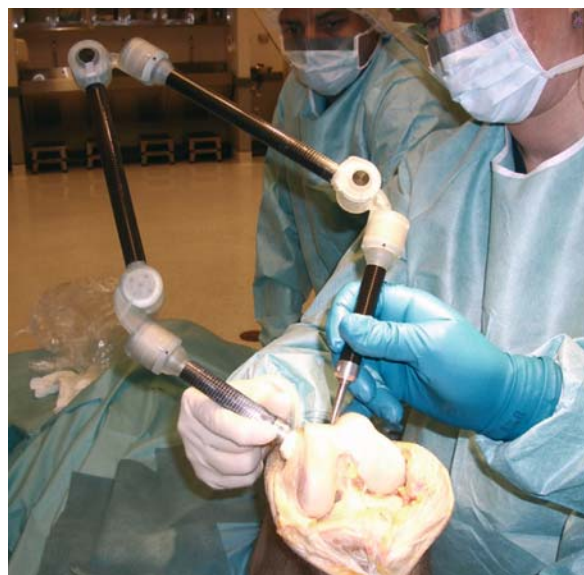
Fig. 78.7. The tip of the linkage is used to digitize the reference points on the femur
