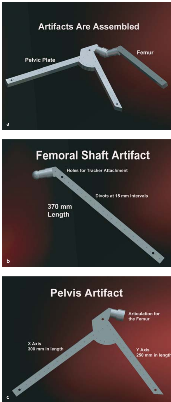
Fig. 9.6. a Phantom or artifact used to assess accuracy of a computer navigation protocol used in total hip arthroplasty. b Details of the femoral shaft artifact. c Details of the pelvic and acetabular artifact. (Figure contributed by Dr Nicholas Dagalakakis, National Institutes of Standards and Technology, Gaithersburg, Maryland)
