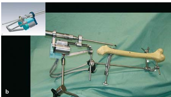
Fig. 75.1a,b. Example of bone mounted robots. a »MBARS« robot positioned for patello-femoral arthroplasty (with permission from Elsevier [9]). b »MINARO« robot positioned for cement removal in revision THA (with permission from Prof K. Radermacher)
