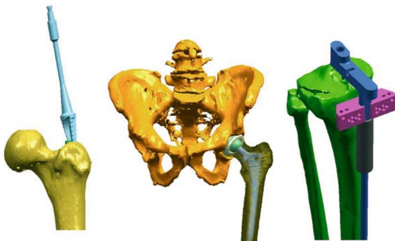
■ Fig. 7.1. 3D representations of instances during surgical procedures showing the relative positions of the patient specific bones and the instruments or components used
