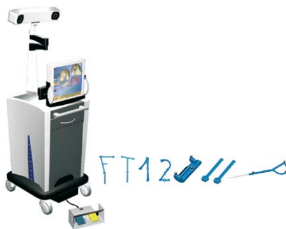
■ Fig. 40.1. Surgetics station and instruments set. F and T reference markers respectively fixed on the femur and on the tibia, 1 and 2 rigidly attached to the classical drill guides
