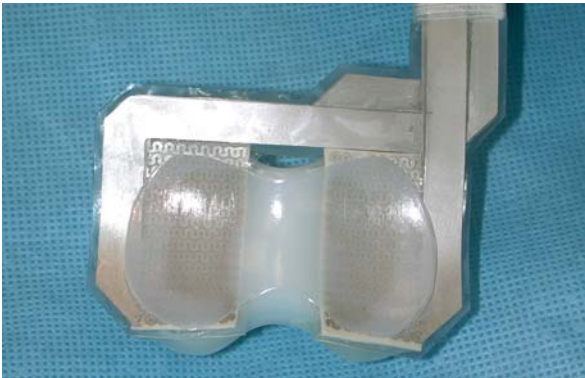
Fig. 23.1. The pressure-sensing device is a modification of a Novel pressure matrix array attached to the upper surface of a tibial polyethylene insert trial. It is sandwiched between the insert trial and a protective low molecular weight polyethylene covering
