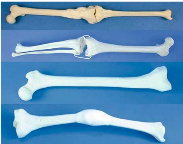
Fig. 69.4. Plastic specimens (Foam Cortical shell, Sawbones, Sweden) with deformities around the knee joint and in the tibial or femoral shafts
