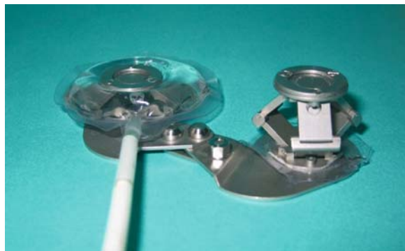
■ Fig. 16.6. Hydraulic prototype shown with fluid-filled pouch and parallel plateau mechanism
