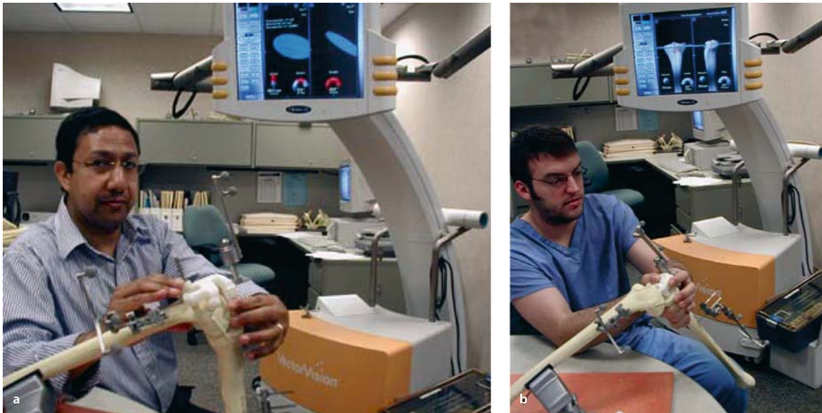
■ Fig. 24.3. Testing the reliability of positioning the femoral (a) and the tibial (b) PST by multiple observers using a navigation system as a measurement tool
