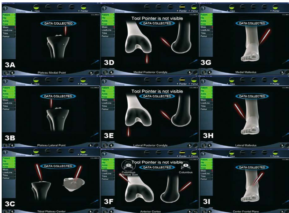
Fig. 4.3a–i. Computer interfaces illustrating position of surface registration pointer necessary to acquire: a–c tibial medial and lateral articular surfaces and tibial mid-point, d,e location of distal femoral articular surfaces and posterior condylar line, f location of anterior femoral cortex, g–i location of center of ankle joint
