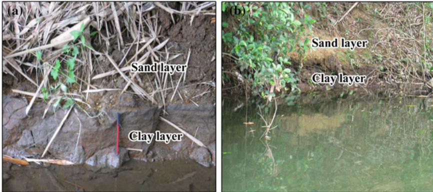
Plate 4.4 Sand and clay layers exposed on the banks of the Manimala river, SW India at two locations. The sand layer exposed on river banks due to bed lowering (channel incision) were once part of the subsurface aquifer system feeding water to the wells in the floodplains. Unfortunately, such movement of water can no longer takes place as the water level has fallen below the permeable (sand) layer
