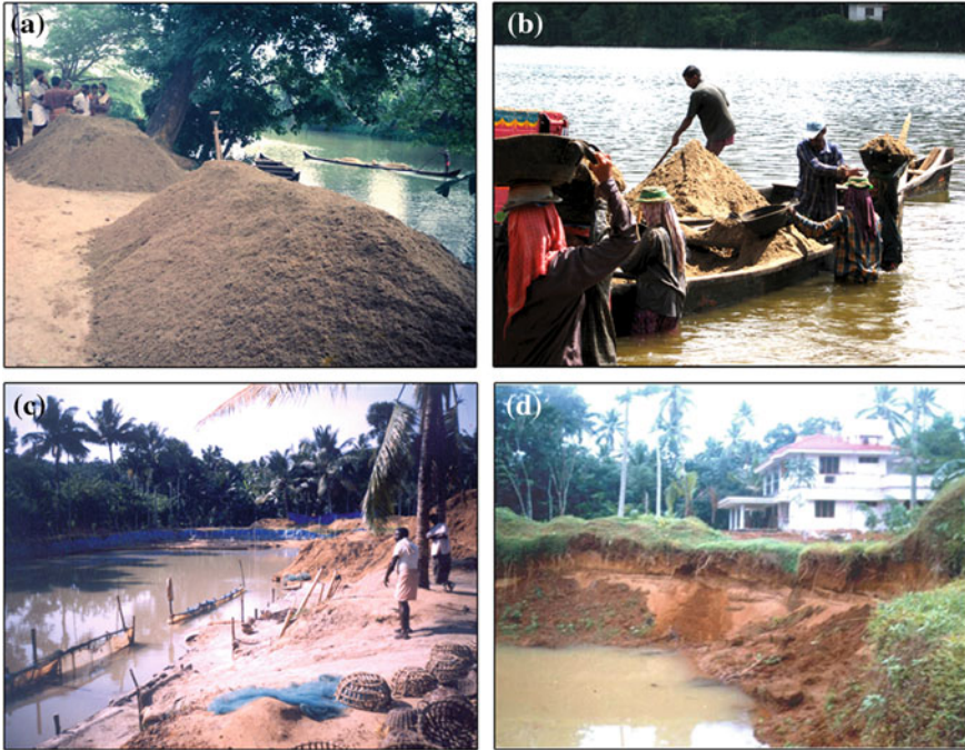
Plate 3.1 Different types of alluvial sand mining. a and b Instream sand mining; c A floodplain sand mine; d Terrace mining under wet condition near the courtyard of a house
