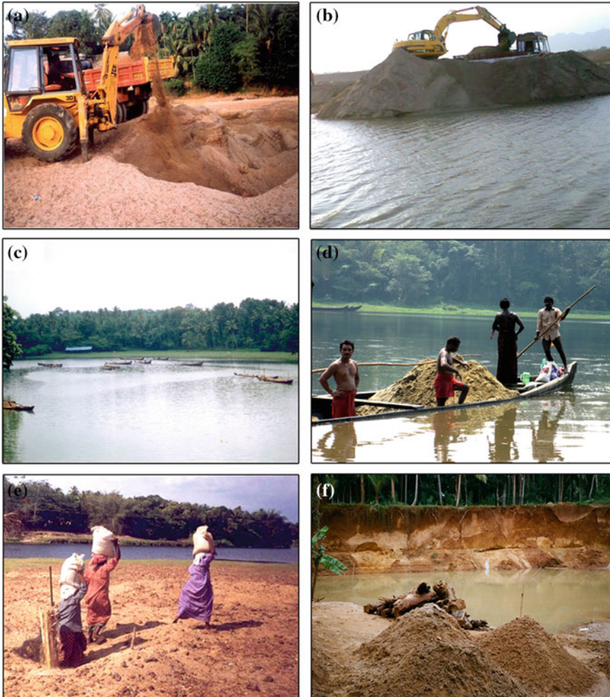
Plate 3.2 Different methods of sand mining. Mechanical sand mining from ephemeral (a) and perennial (b) rivers; Manual mining from active channels (c, d); Manual mining from point bar deposit (e); Wet pit mining from floodplain (f)
