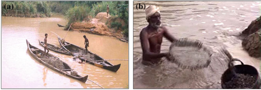
Plate 4.7 Mud water rivers! Many small rivers in the southwest coast of India (at their storage zones) became mud water rivers because of high load of particulate matters derived from sand mining close to river banks (a) and washing of clayey sand (low grade sand) for improving their quality (b)
