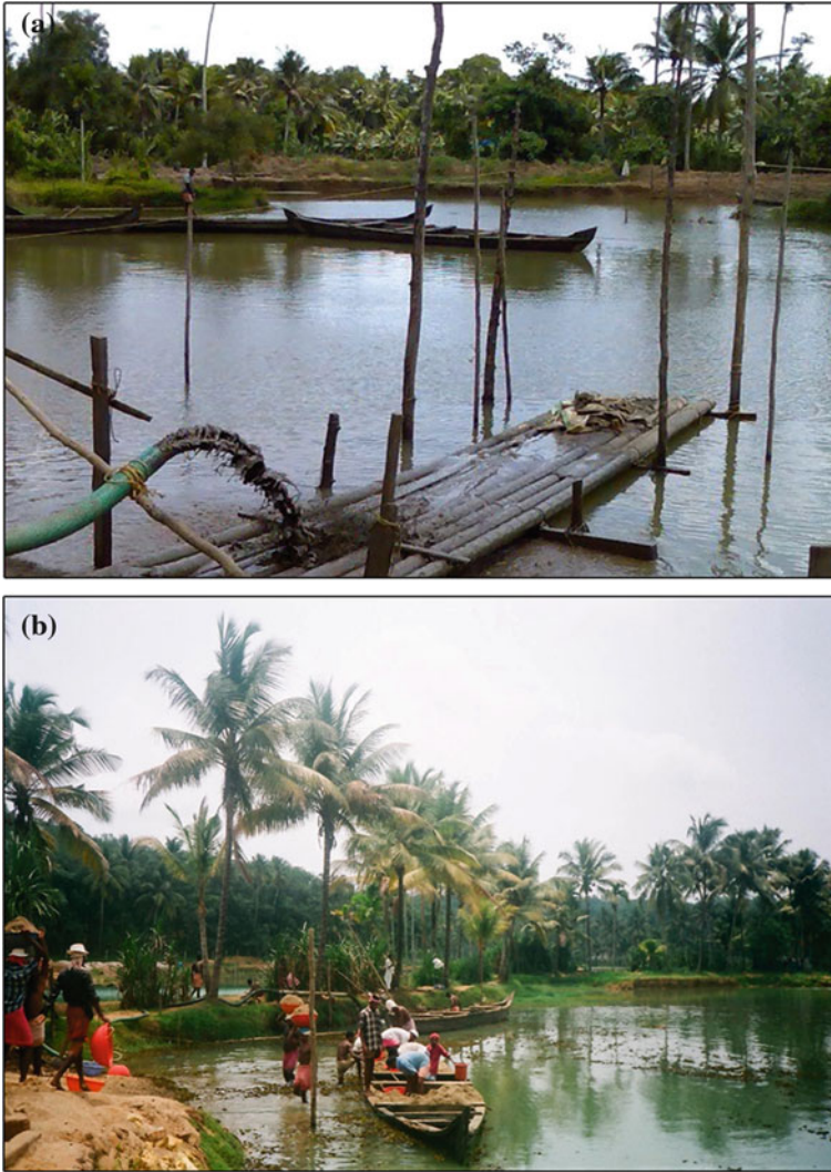
Plate 5.3 Mechanised (using high power jet pump) and manual floodplain mining from the coastal lowlands of Muvattupuzha river basin, Southwest India
