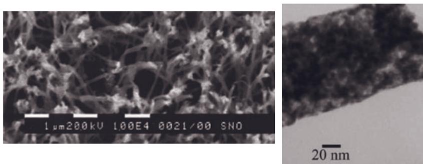
**Figure 6.11** Fiber-like  $\text{SnO}_2$  nanostructured anodes. (Reproduced from Ref. [22].)
