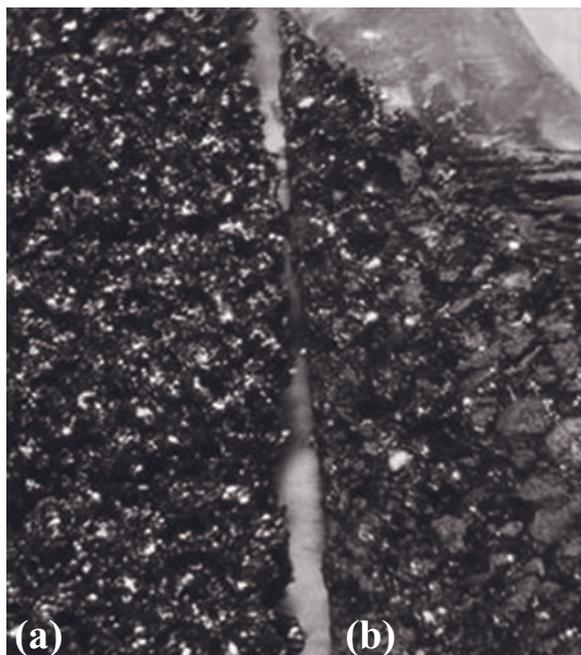
**Figure 3.7** Microcell™ foams do not experience mechanical damage during electrochemical cycling. (a) An uncycled Microcell™ foam, (b) Microcell™ foam after usage; taken from [6].
