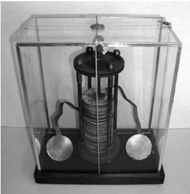
**Figure 2.2** An illustration of Volta's cell, called a "Voltaic Pile"; taken from [3].
