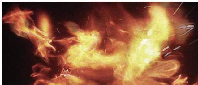
**Figure 4.8** One safety concern is the ignition of gases released from overcharged batteries that can produce flame clouds [18].
